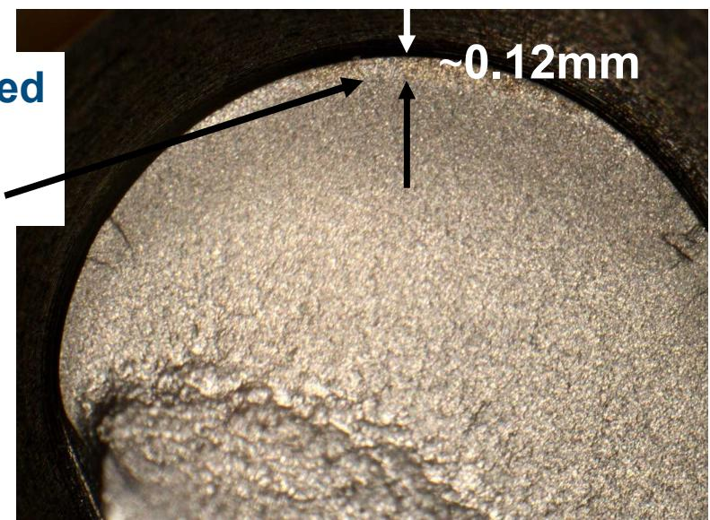
Crack lengths  $<10\mu\text{m}$  can be resolved with DCPD
