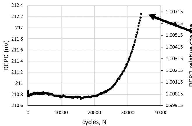
Test interrupted and then heat tinted
