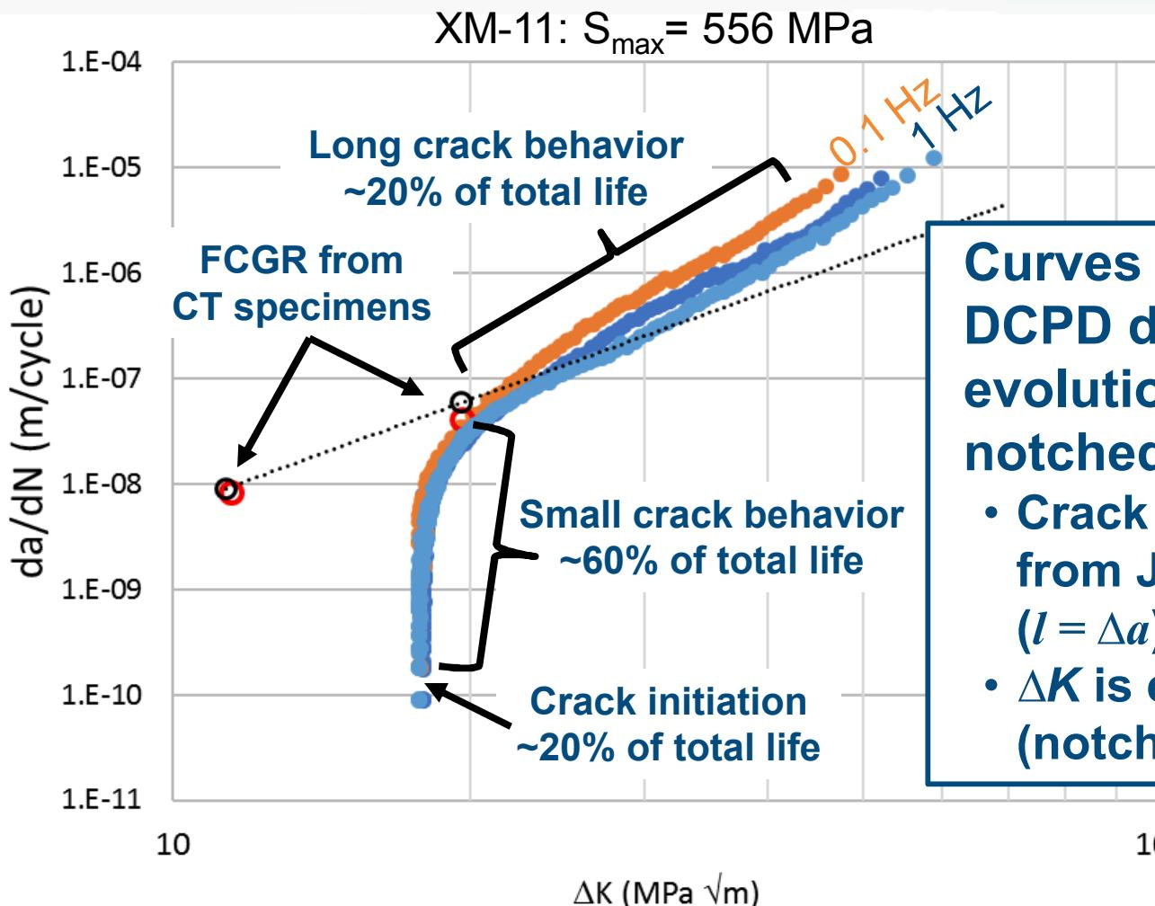
Curves are derived from DCPD data to track crack evolution during fatigue of notched specimens
