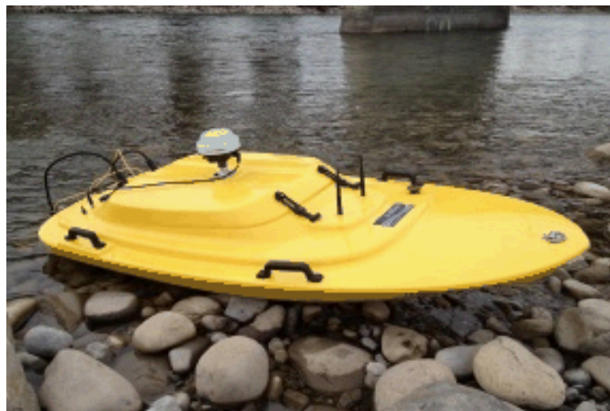
Remote control boat with RTK GPS
