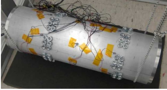
a) Aluminum nuts clustered around cylinder to add mass.
