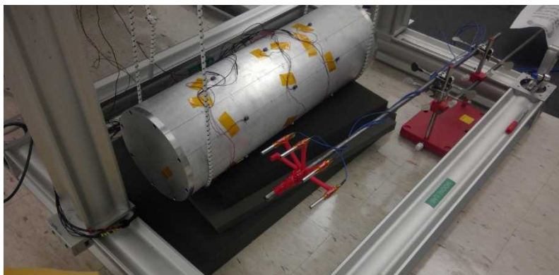
a) Cylinder suspended from soft bungee cords with the accelerometers bonded on the outer surface, and the microphones distributed in an array.
