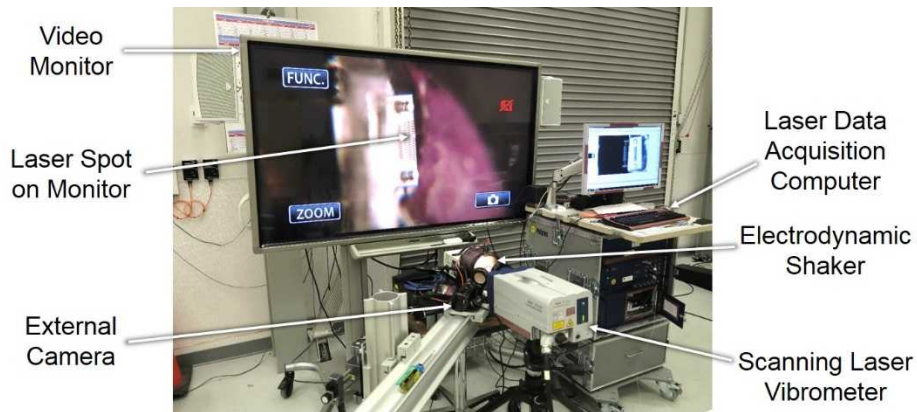
Figure 5: Overview of test setup showing the laser vibrometer, shaker, and video monitor used to find the laser spot.
