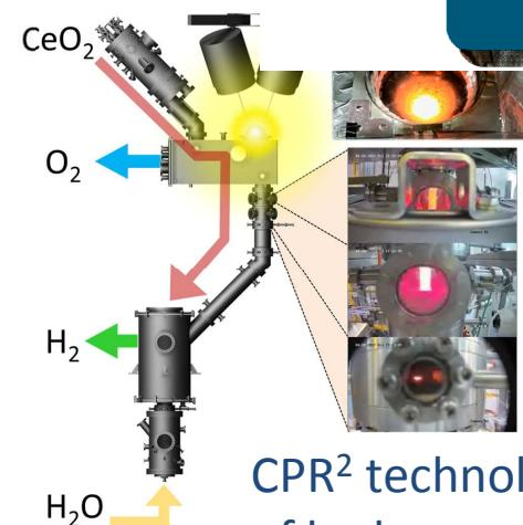
CPR<sup>2</sup> technology produced 2 liters of hydrogen on simulated sun.
