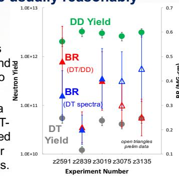
**Using a cylindrical geometry and deuterium fuel allow us to diagnose fuel magnetization at stagnation.**
