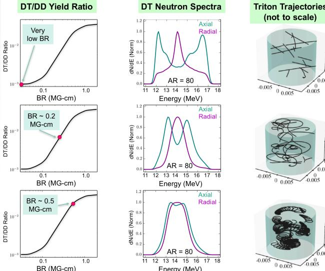
**Asymmetry in the secondary DT neutron spectra is due to the cylindrical geometry.**
