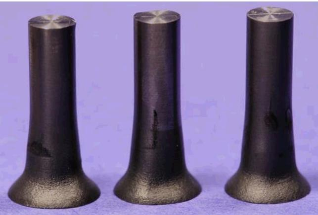
*Taylor cylinder impact testing to validate strength models.*
