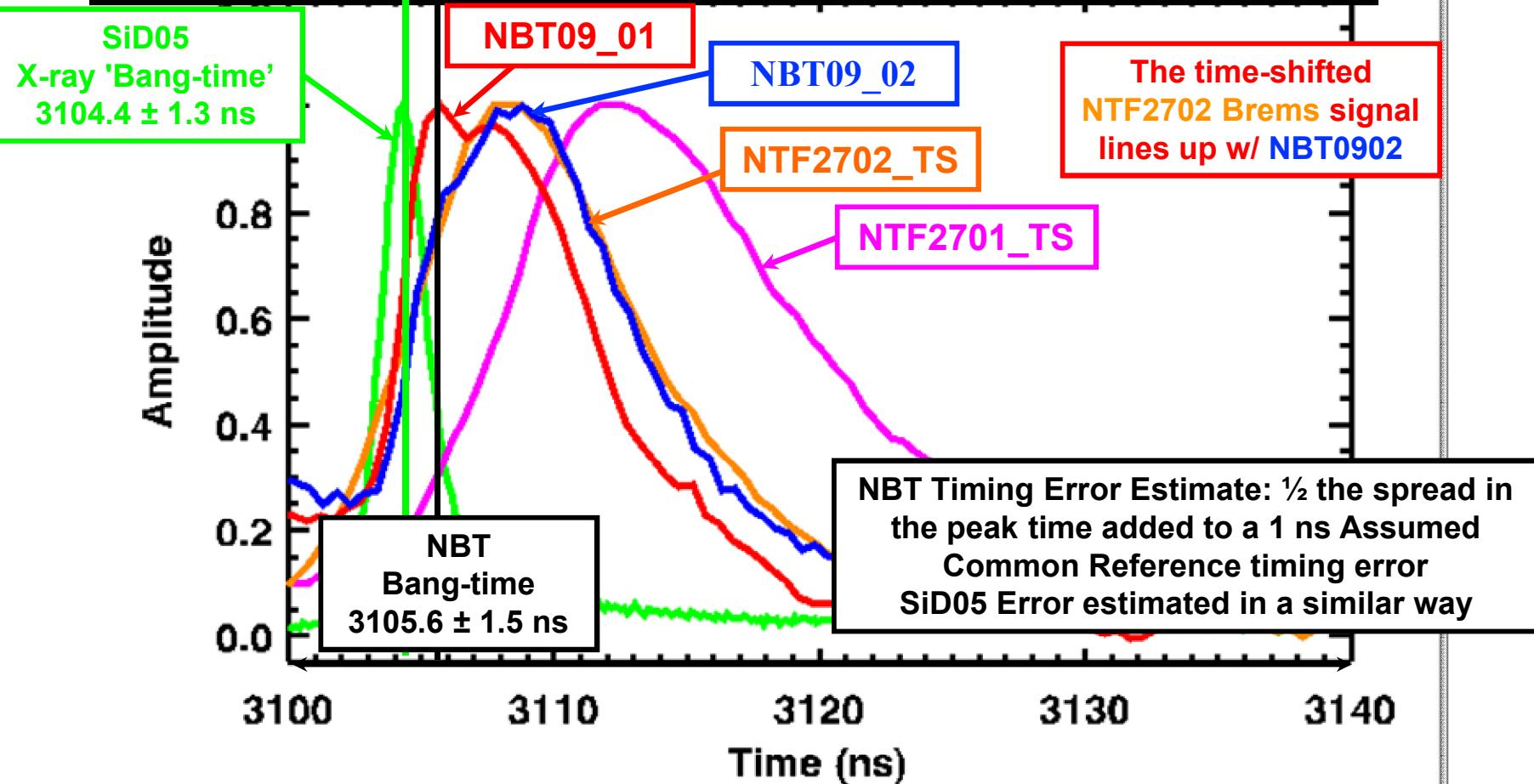
Detector throughput taken into account assuming 0.3 ns plus detector rise-time of  $\sim 0.65$  ns
