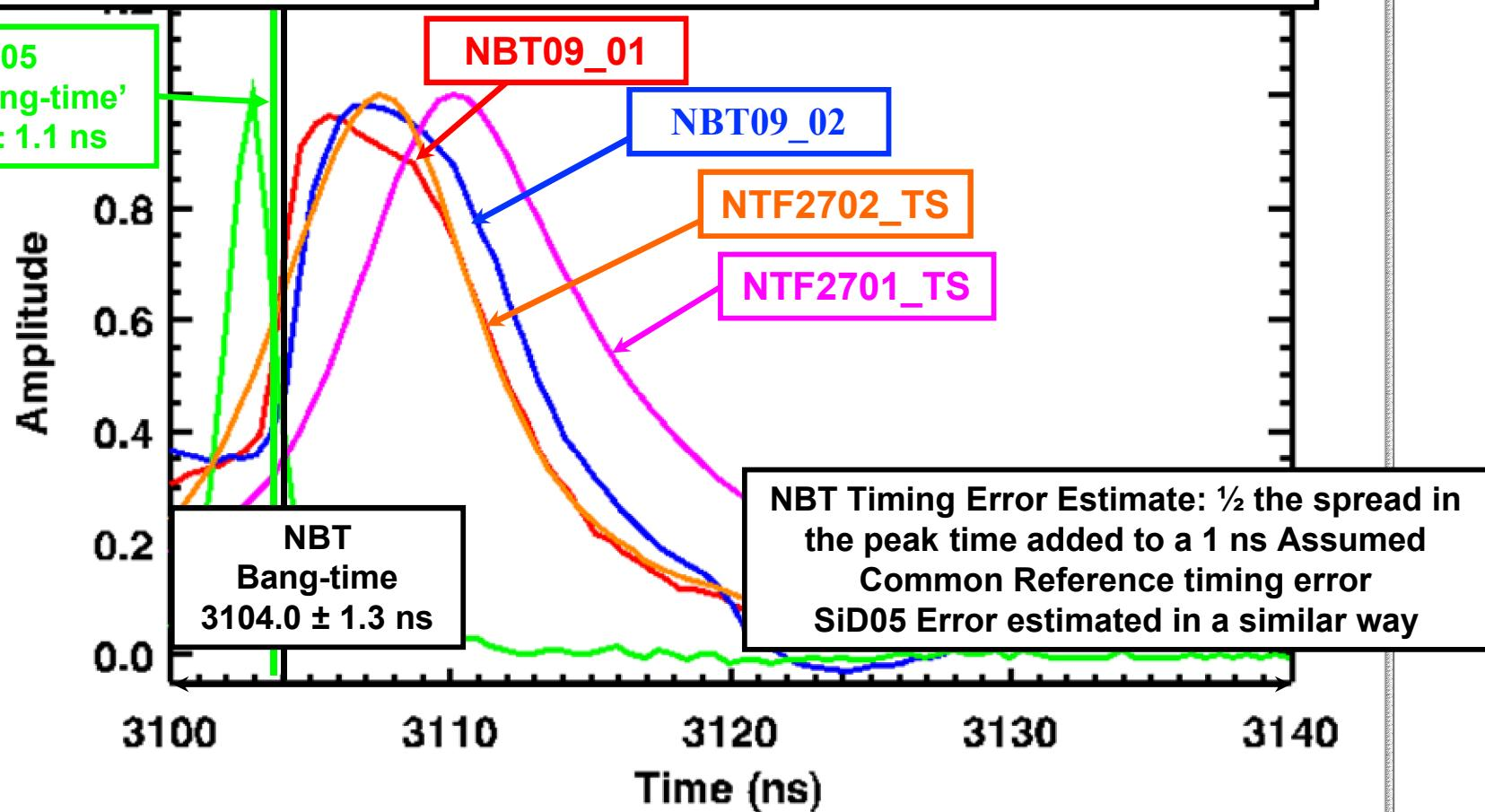
Detector throughput taken into account assuming 0.3 ns plus detector rise-time of  $\sim 0.65$  ns
