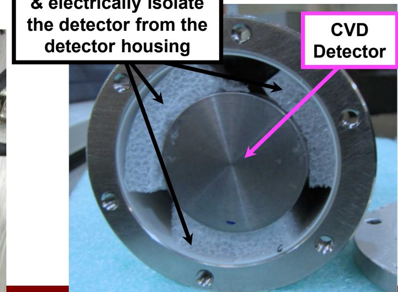
In this low noise setup a  $\pm 5\text{mV}$  bit noise limited signal was obtained on MagLIF Shot 3157 with a DD yield of  $\sim 6\text{E}11$
