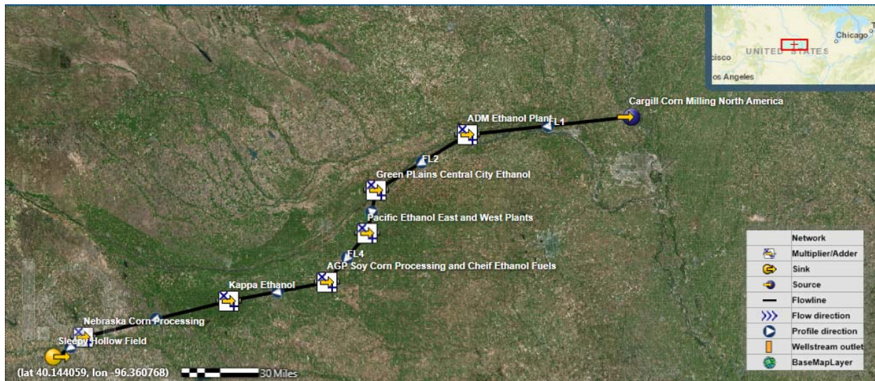
Figure 6-6. PIPESIM pipeline model showing an approximate route and related ethanol CO 2 sources
