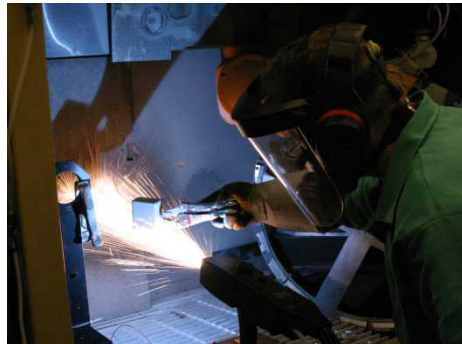
Twin Wire Arc Spray
