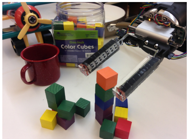
Fig. 1: PCF-sensors on a Baxter parallel gripper. Seven infrared sensors are spaced along each finger’s contact area, and one is mounted at each tip for object detection and force control
