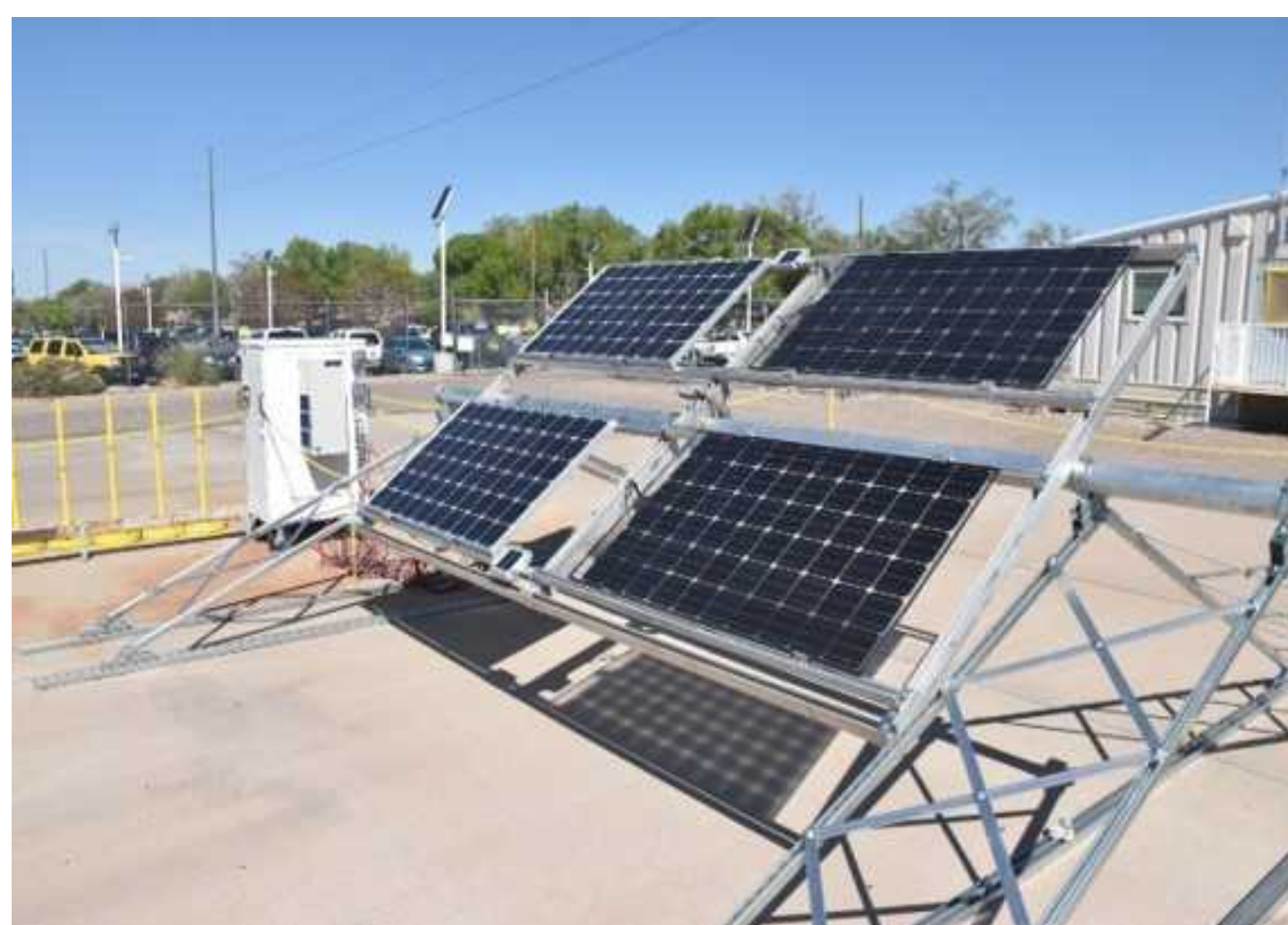
Adjustable rack for measuring bifacial module performance at various tilts and heights.
