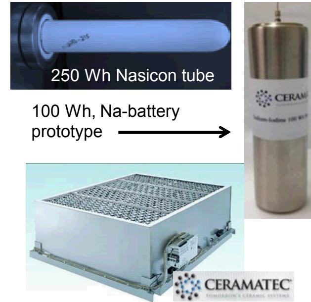
Ongoing efforts targeting for large scale (10kWh), intermediate temperature demonstrations (w/ Ceramatec: 180 Wh/l, \$150/kWh, 2.6V, 40 cells).
