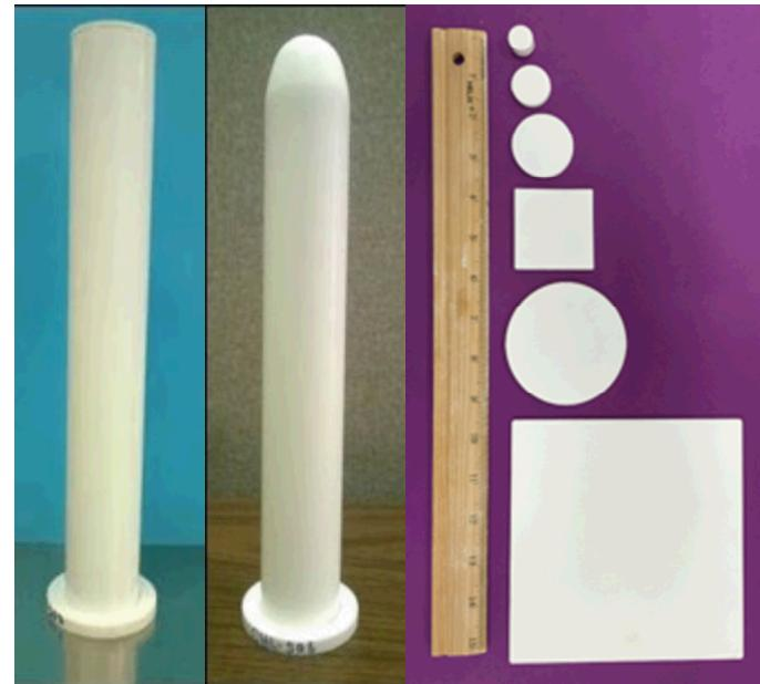
Engineered materials chemistry and advanced, scalable processing (Ceramatec, CoorsTek) make NaSICON a *chemically/mechanically stable, low temperature, high conductivity (>10<sup>-3</sup> S/cm @RT) separator technology.*
