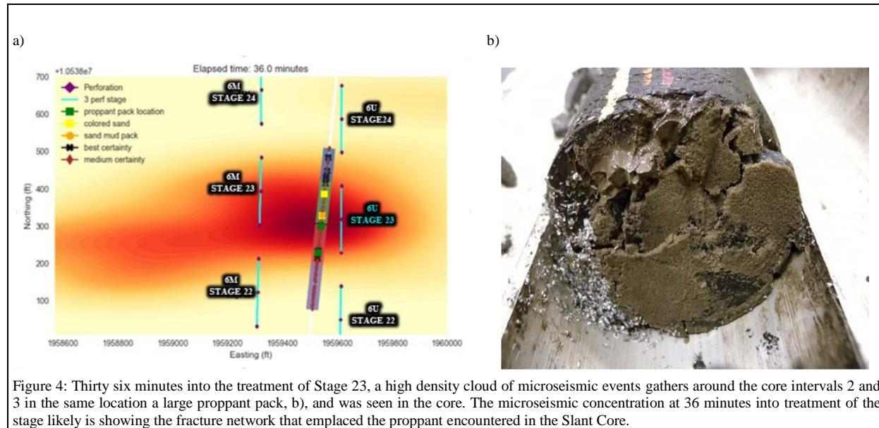
Figure 4: Thirty six minutes into the treatment of Stage 23, a high density cloud of microseismic events gathers around the core intervals 2 and 3 in the same location a large proppant pack, b), and was seen in the core. The microseismic concentration at 36 minutes into treatment of the stage likely is showing the fracture network that emplaced the proppant encountered in the Slant Core.
