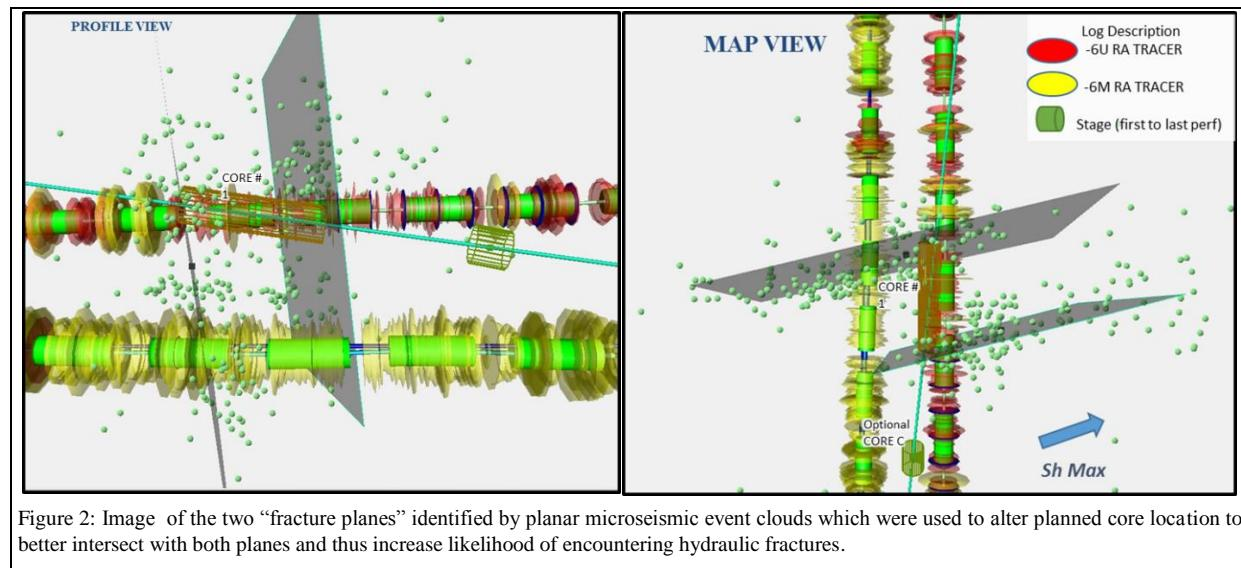
Figure 2: Image of the two “fracture planes” identified by planar microseismic event clouds which were used to alter planned core location to better intersect with both planes and thus increase likelihood of encountering hydraulic fractures.
