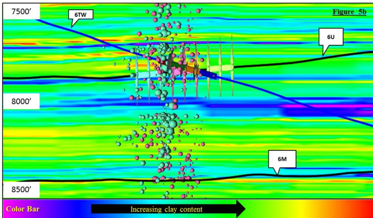
Figure 5a Proprietary geocellular model of calcite volume. Figure 5b: Proprietary geocellular model of clay volume. On both figures, notice the arresting of events in the center of the figure coinciding with elevated calcite/lower clay volume. The cyan microseismic events are from Stage 24, purple events are Stage 23.
