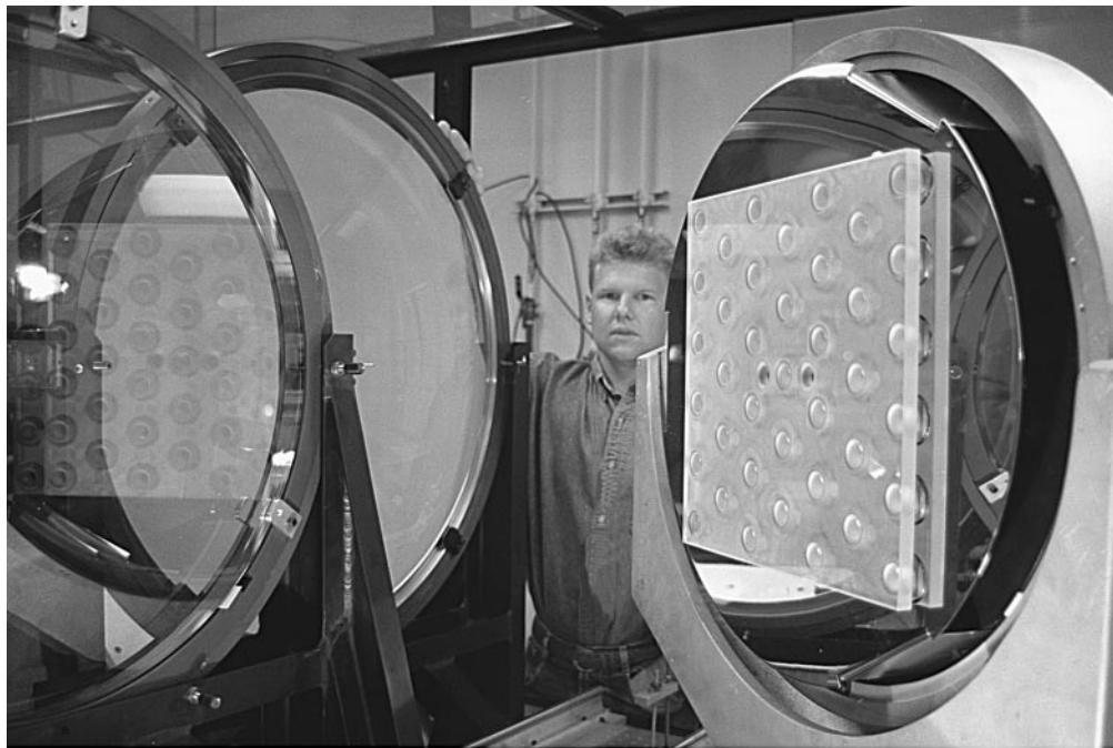
large-aperture mirrors using different methods of actuation. These mirrors will be tested at LLNL in 1998.
