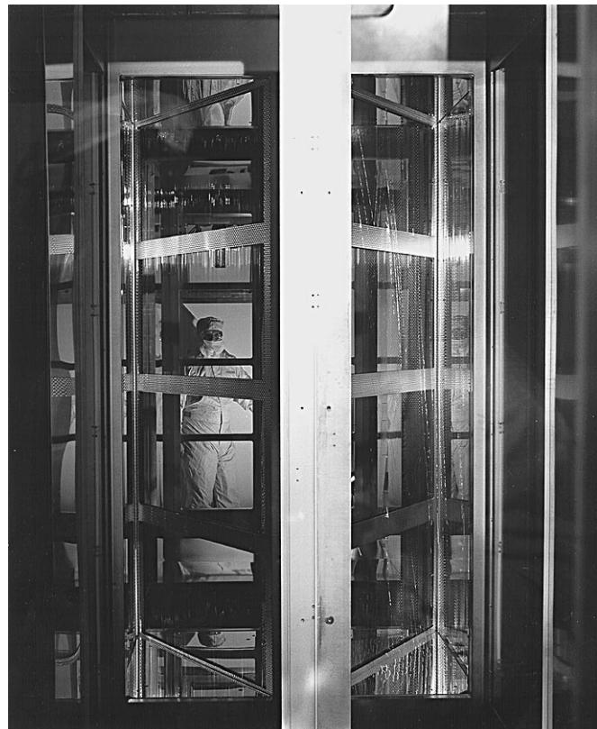
FIGURE 7. NIF prototype amplifier under test in AMPLAB.
