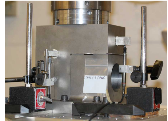
Quasistatic Shear Test Setup
