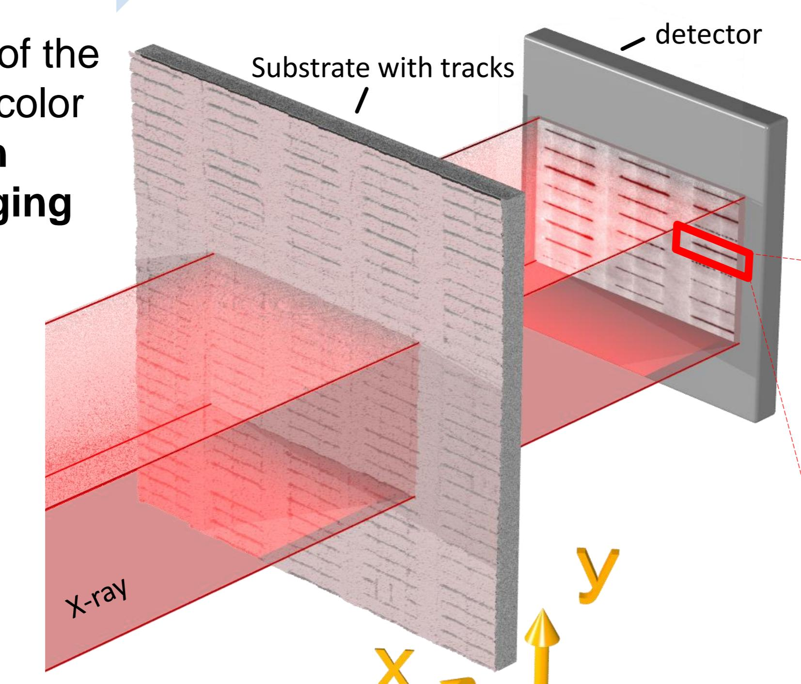
4) **Image processing and pores detection using x-ray radiography**
