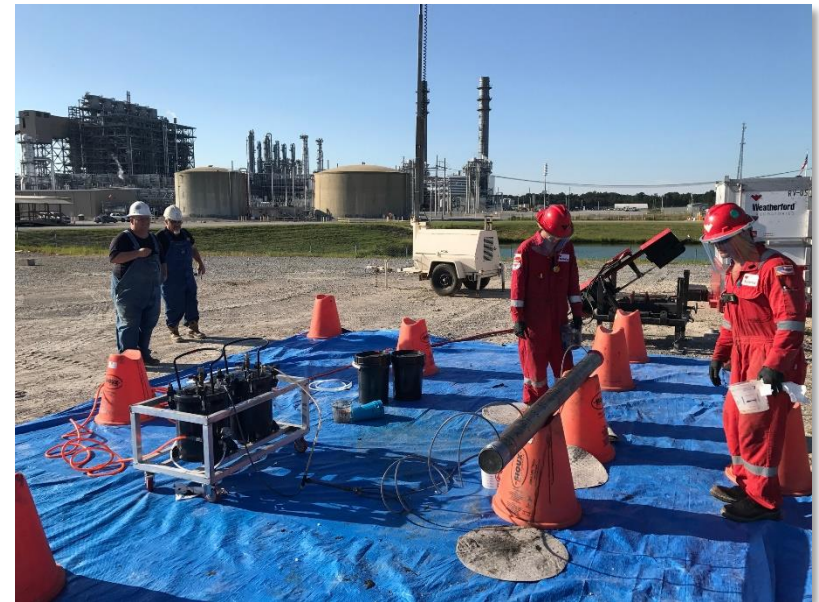
MPC 10-4 Epoxy injection for core preservation
