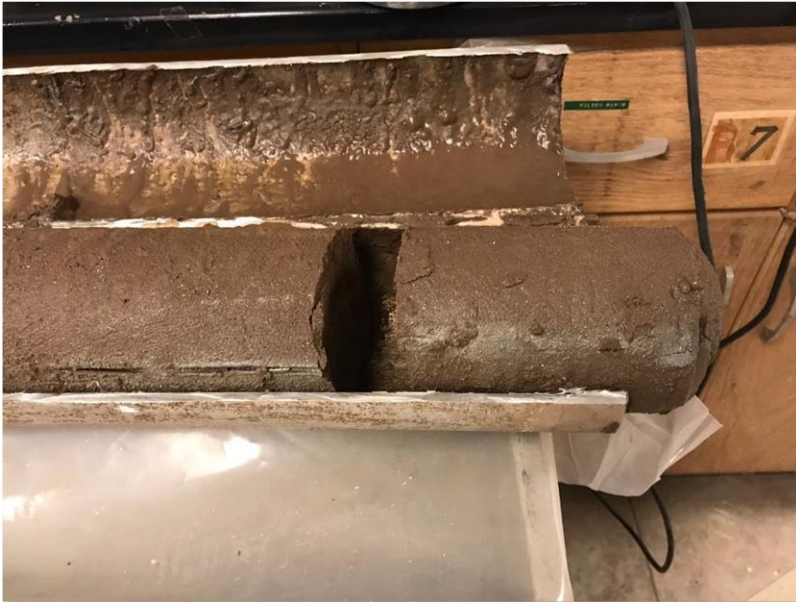
MPC 26-5 Lower Tuscaloosa massive – very poorly indurated sandstone, well caked
