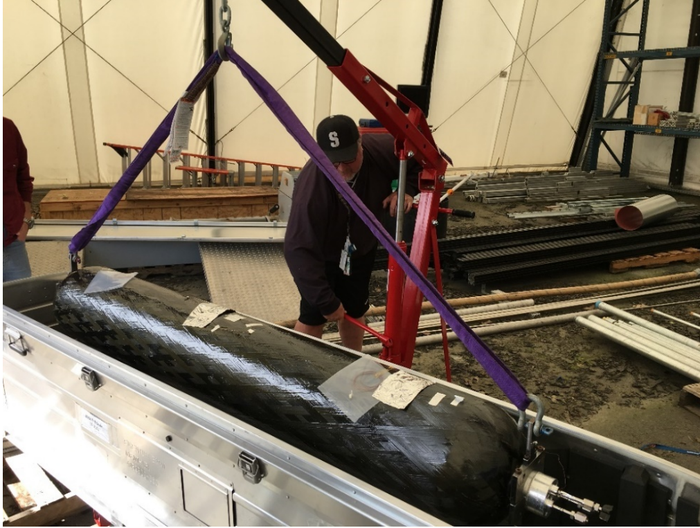
Figure 8: Prototype pressure vessel being extracted from shipping container
