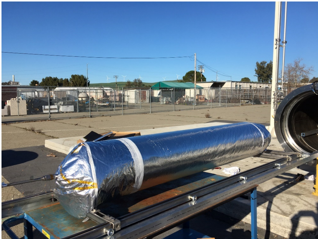
Figure 9: Prototype pressure vessel wrapped with ~10 layers of MLI, prior to being inserted into containment vessel
