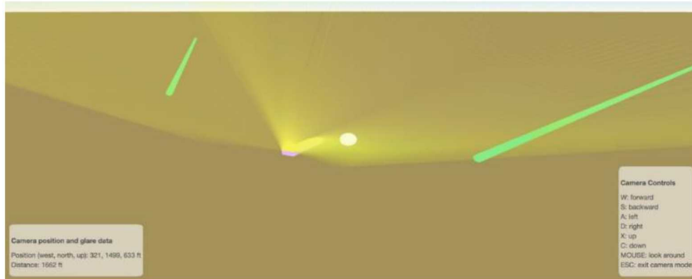
Figure 7. Glare Visualization of MHT array (purple) with Air Traffic Control Tower (white), flight path (green), and cumulative daily glare for July 1.
