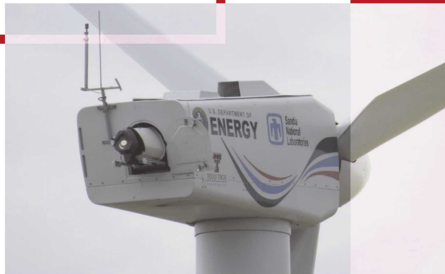
SpinnerLidar instrument installed on a SWiFT turbine. The instrument produced the wake measurement data used for wake dynamics analysis.
