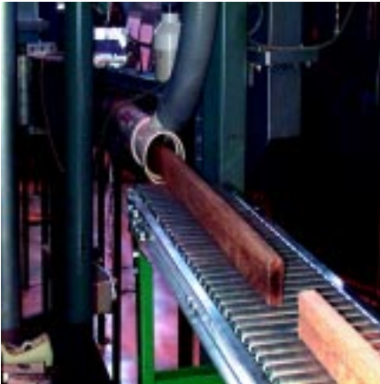
Lumber undergoing microwave drying at ORNL.
