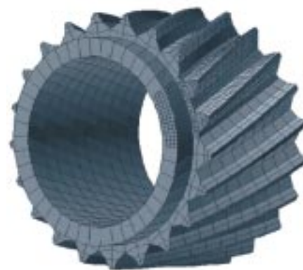
Meshed shape used to simulate a helical gear.
