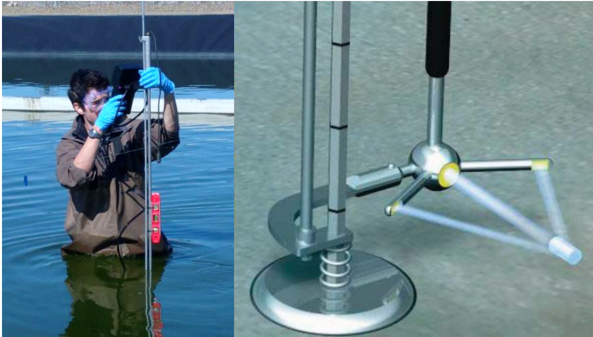
Figure 73: (left): Reading x and y velocity from the Sontek Flowtracker. (right): Visualization of the Sontek Flowtracker Acoustic Doppler Velocimeter. Reprinted from “Automated Quality Control in the SonTek® FlowTracker®”, by SonTek, Retrieved December 12, 2015, from https://ysi.actonsoftware.com/acton/attachment/1253/f-0163/1/-/-/-/-/Automated%20Quality%20Control%20in%20the%20SonTek%20FlowTracker%20-%20SmartQC.pdf . Reprinted with permission.
