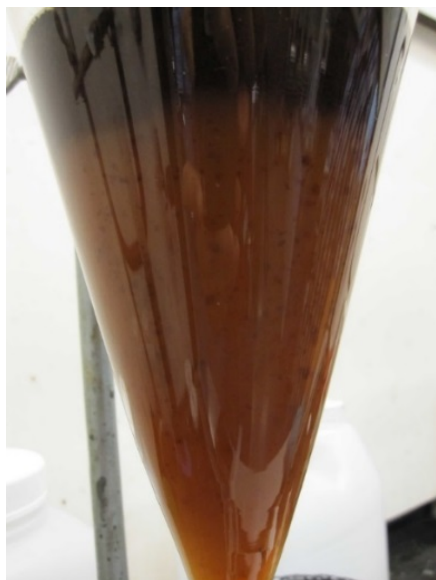
Figure 105: Sample 1 Oil-Water Phase Separation
