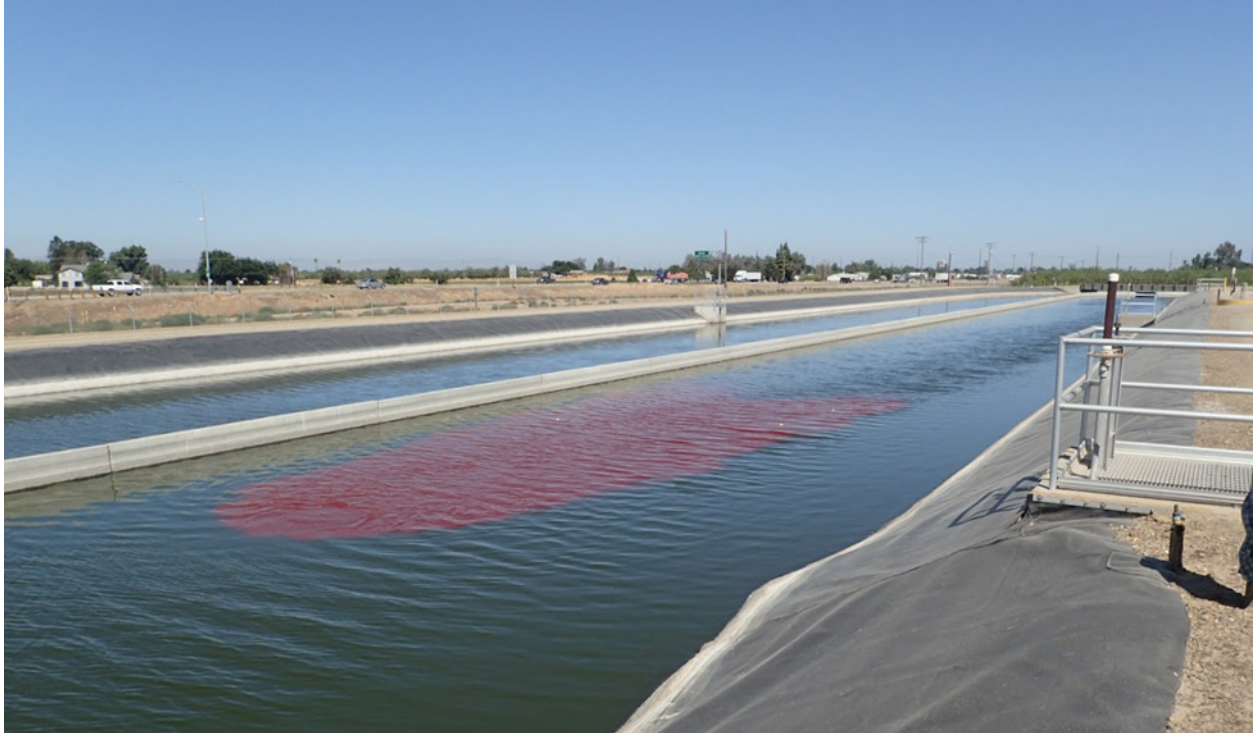
Figure 75: Tracer plume addition to the inner raceway via the weir box at right. Influent is piped underground and upwells at mid-width of the channel.
