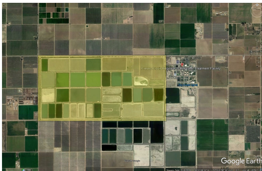
Figure 121: An aerial image of the Fresno-Clovis Regional Wastewater Treatment Facility. As shown, the facility is surrounded by open agricultural land. A 500-ha lot is highlighted to demonstrate a hypothetical location for the collocated algae biofuels production facility.
