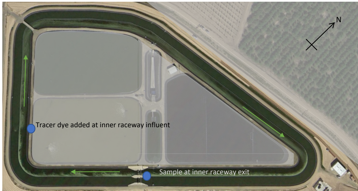
Figure 74: Tracer experiment injection point, flow direction, and sample point.
