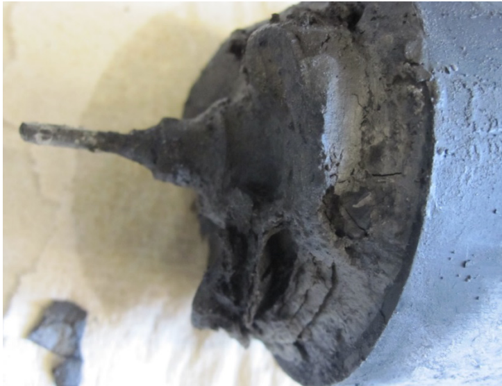
Figure 110: Mineral Encrusted CSTR Paddle
