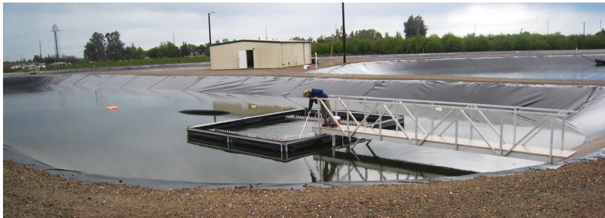
Figure 29: Sampling of the ASP over the overflow weir.
