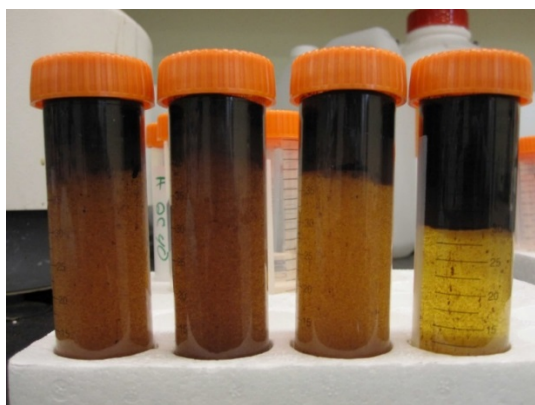
Figure 106: Sample 1 Oil-Water Partition in Centrifuge Tubes
