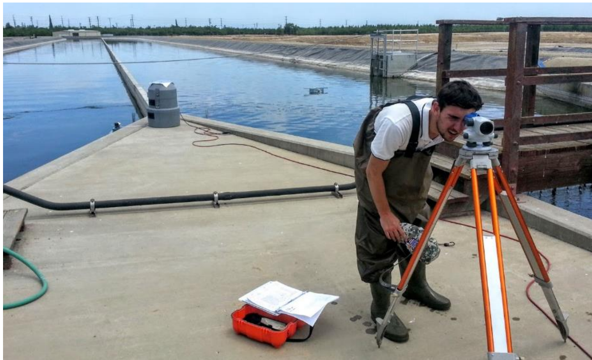
Figure 72: Differential leveling to measure head loss (i.e., paddle wheel lift) as change in water surface elevation before and after the paddle wheel.
