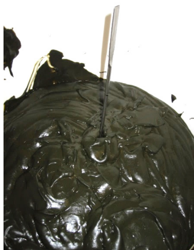
Figure 84: Sample 2 Homogenized, 17.6% Solids Feedstock
