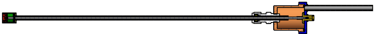
Figure 4: Schematic of new fission chamber. The detector body shown in Figure 4 is on the far left. The pressure gauge and fill valve would be on the far right.
