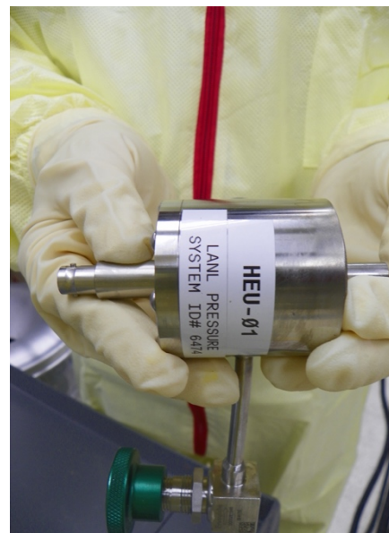
Figure 11: Mark II Fission Chamber loaded with an HEU reference foil.
