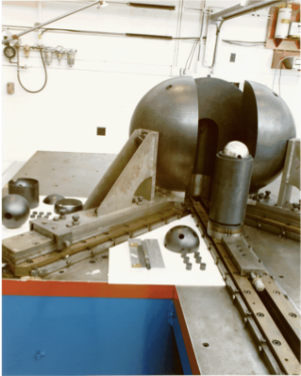
Figure 1: Photograph of the Flattop-HEU assembly at TA-18.
