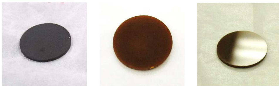
Figure 8: BCZY18 membrane pellets, (a) synthesized at Sandia and (b, c) from Colorado School of Mines. The image in (c) shows the reflection of the fluorescent light, an indication of the high density of the pellet.
