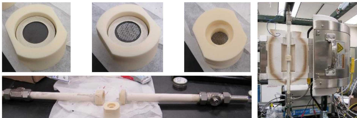
Figure 4: Assembly of membrane cell (Top) and test cell (Bottom). Right: assembled test cell plumbed and in furnace.
