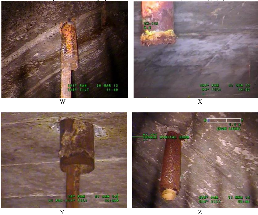
Figure 6-1: Pictorial Definitions of Degrees of Corrosion (RPP-RPT-55951) (6 sheets)
