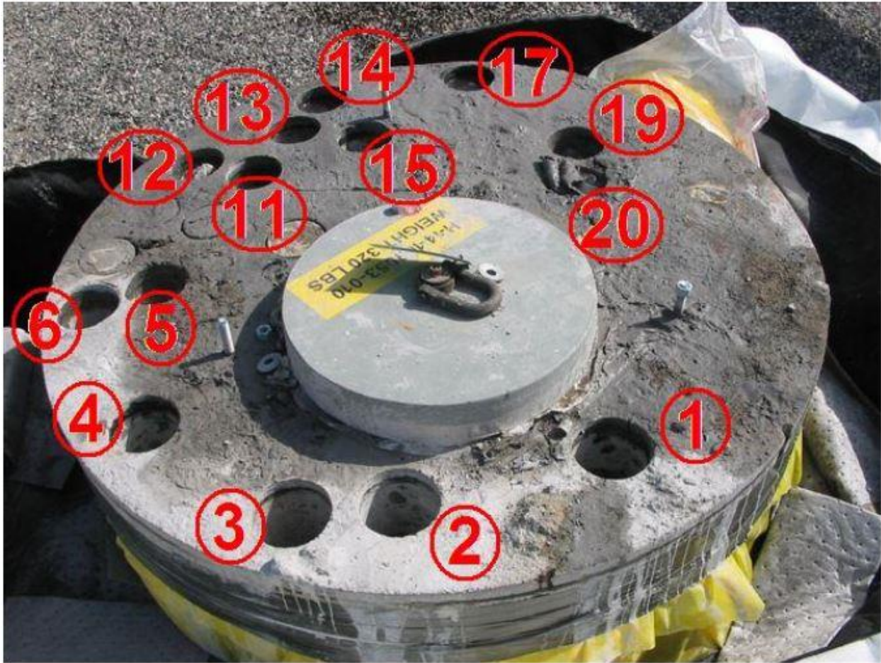
Figure 4-36: Concrete Plug with the Cores Removed (RPP-RPT-50934)
