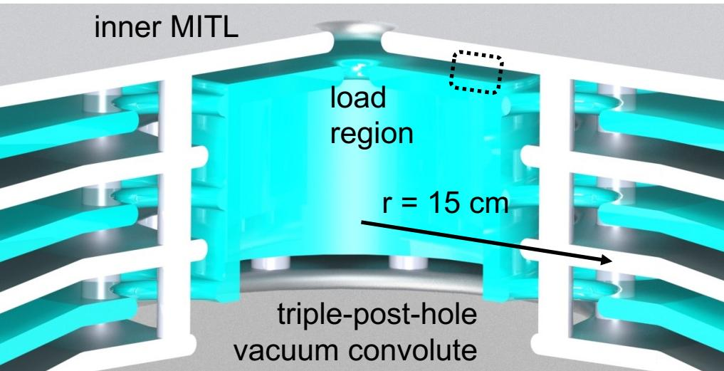
six outer magnetically insulated vacuum transmission lines (MITLs)
