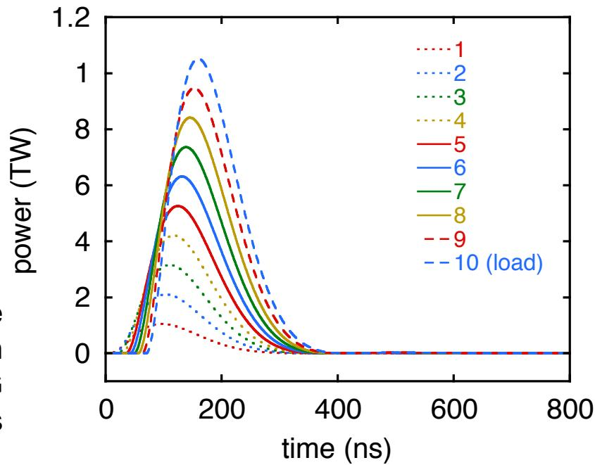
10-stage IMG module with 20 bricks per stage
