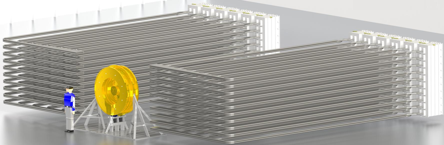
**Neptune stores 11 MJ of electrical energy, generates a peak electrical power of 50 TW, and delivers an arbitrary pressure-loading time history to a material-physics load.**
