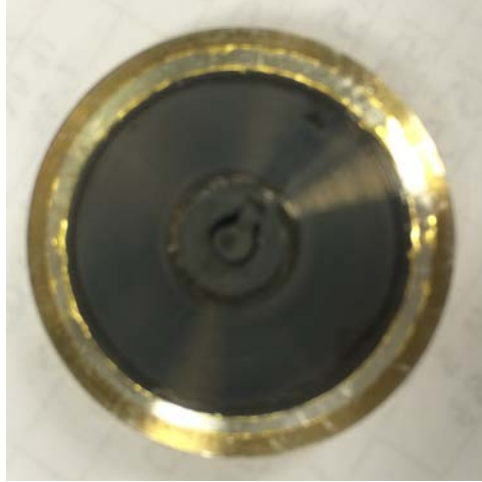
Figure C1: Photo of the 24 hour electron-beam irradiated T91 in 3 ppm H 2 saturated water.
