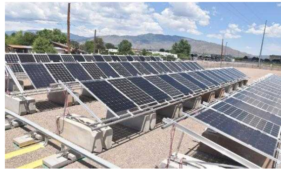
Figure 3: String-level bifacial and monofacial test array in New Mexico.
