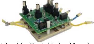
Fig. 16. Fabricated module with gate drive board for evaluating the effect of L_{middle} during switching transient.
