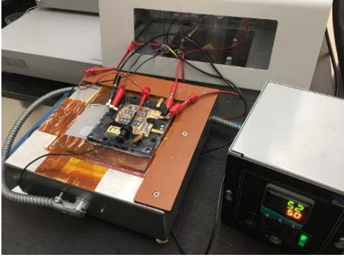
Fig. 6. The test set up for static characterization of the 1200 V SiC Trench MOSFET module.
