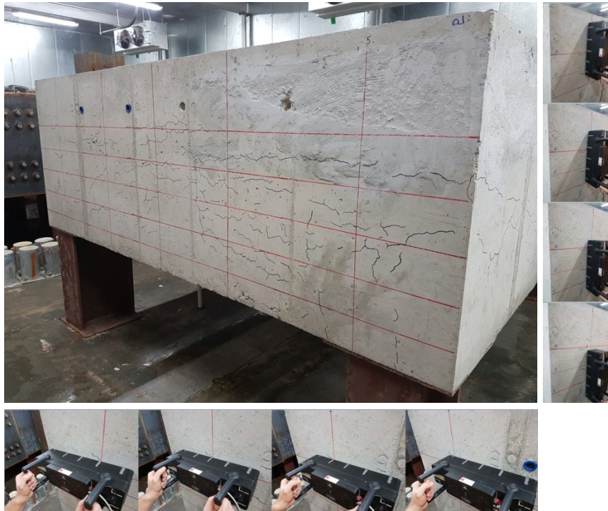
Figure 6. Lateral surface grid with lateral MIRA measurements on line A and horizontal MIRA measurements on line 1.
