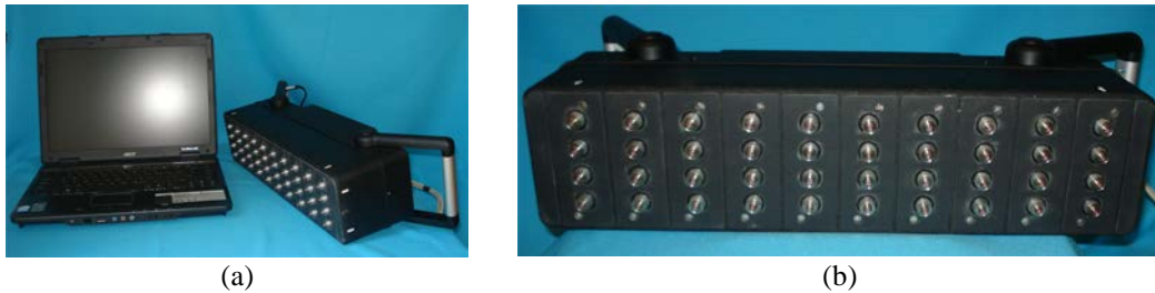
Figure 4. (a) MIRA version 1 system. (b) MIRA version 1 ultrasonic array face. (Images courtesy of Germann Instruments, Inc.).
