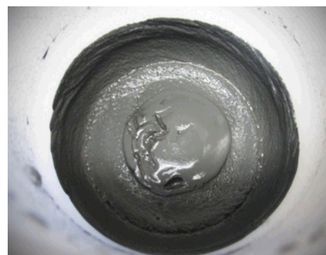
Fig. 11 ~56 vol % B 4 C suspension after pH adjusted to >9
