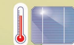
**4. Cell Temperature** – Cell temperature is influenced by module materials, array mounting, incident irradiance, ambient air temperature, and wind speed and direction.
