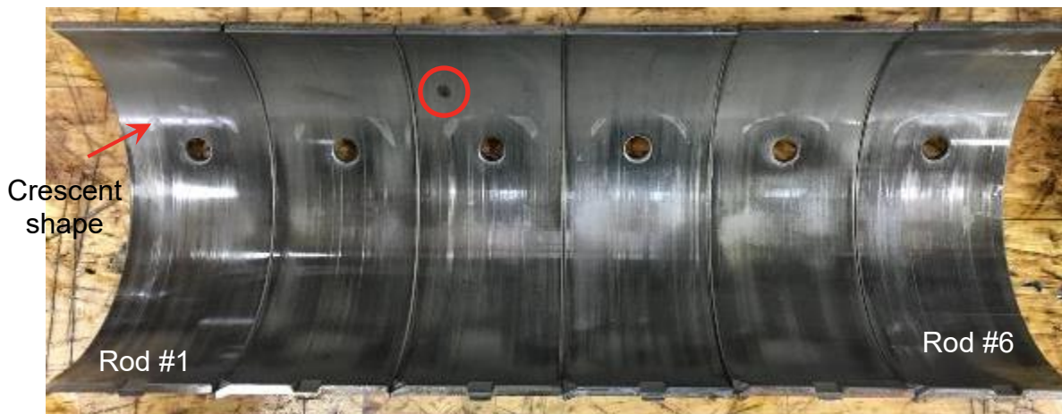
Figure 196: The upper rod bearings after the tests with the low HTHS oils. Cavitation can be seen in a crescent shape around the oil hole. There's also a deep mark on rod #3 breaking from debris.
