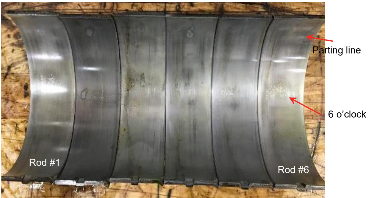
Figure 195: The lower rod bearings after the tests with the low HTHS oils. Cavitation and pitting can be seen at the 6 o'clock position and at the parting line.
