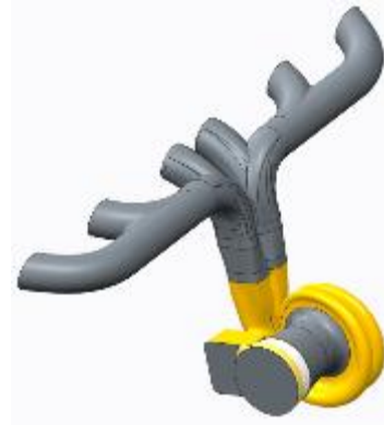
Figure 35: ISX 1999 Manifold (TB1436) and B84 dual inlet Turbo flow geometry
