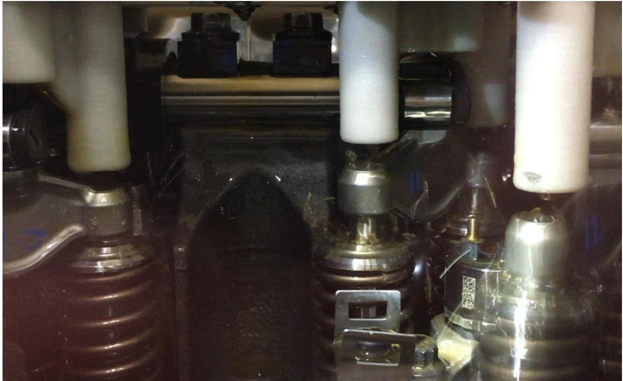
Figure 21: Oil dripping at various moving joints at 1400 engine RPM
