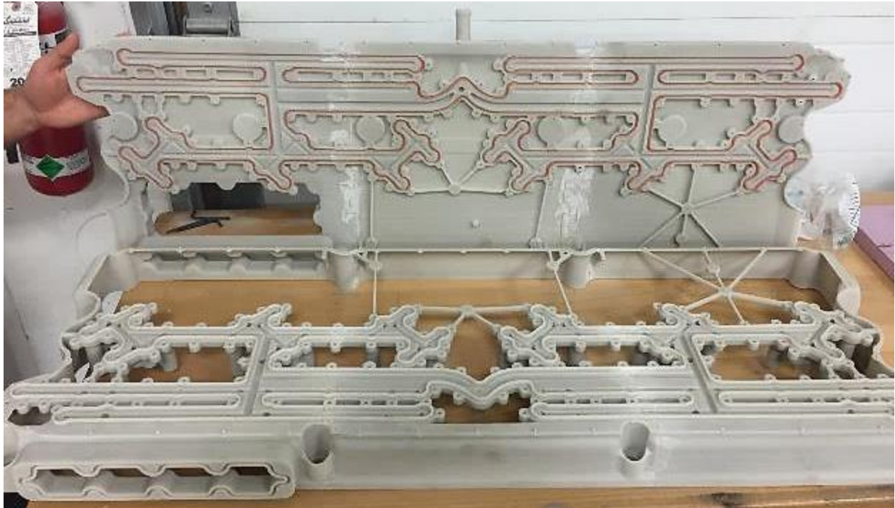
Figure 12: 3D printed valve cover with sections showing the internal oil feed circuit
