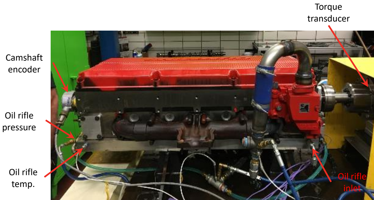
Figure 181: The baseline 2017 ISX 15L cylinder head on the 75hp rig at the Mechanical Efficiency Lab.
