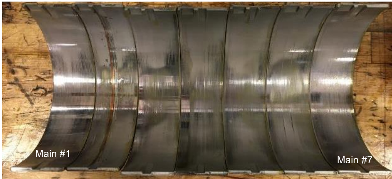
Figure 193: The lower main bearings after the tests with the low HTHS oils. There is a deep score in the main #2 bearing from debris.
