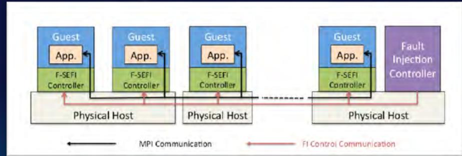
FSEFI v3 adds capabilities for tracing fault corruption as it moves inside a process and across processes in a parallel application
