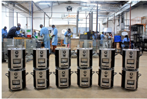
Figure 31. Image of stoves G35B prototype stoves fabricated by Devin Udesen at the Burn Design Labs Nairobi factory. These stoves are being distributed to rural Kenyan households and will be measured for performance by Berkeley Air Monitoring
