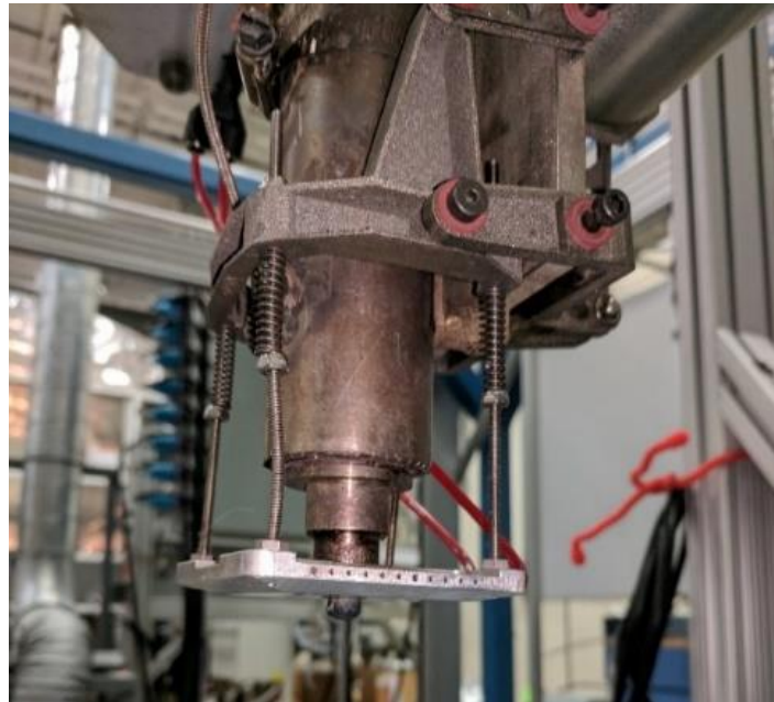
Fig 1. Omnidirectional BAAM-type (Big Area Additive Manufacturing) polymer printing head.
