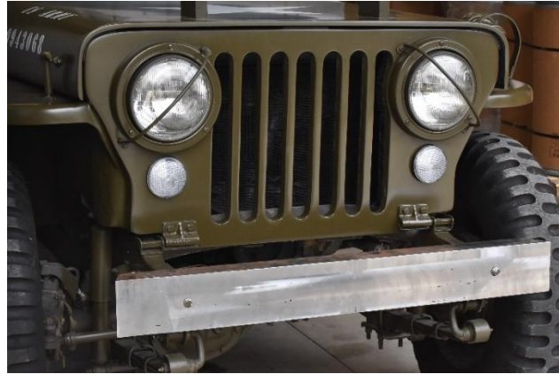
Fig. 12 Willys Jeep with a 3D printed bumper.
