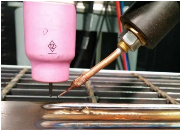
Fig. 2 Directional GTAW (TIG) deposition head with right side forward feeding wire.
