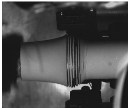
Cracks evident in rings 24 us after impact
