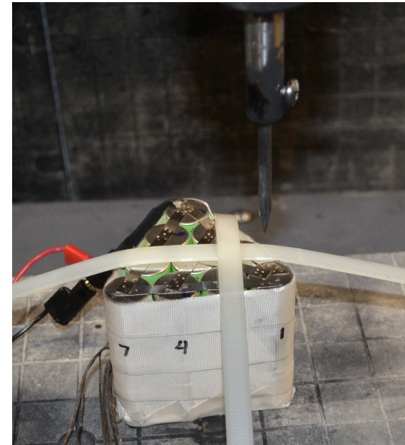
1S10P Battery: Failure point on edge cell
