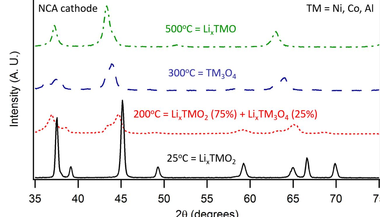
NCA cathode decomposition takes place below 200°C with  $Li_xTMO_2$  releasing  $O_2$  and heat, turning into  $Li_xTM_3O_4$ . Cathode involvement is likely responsible for  $HR_{max}$ .
