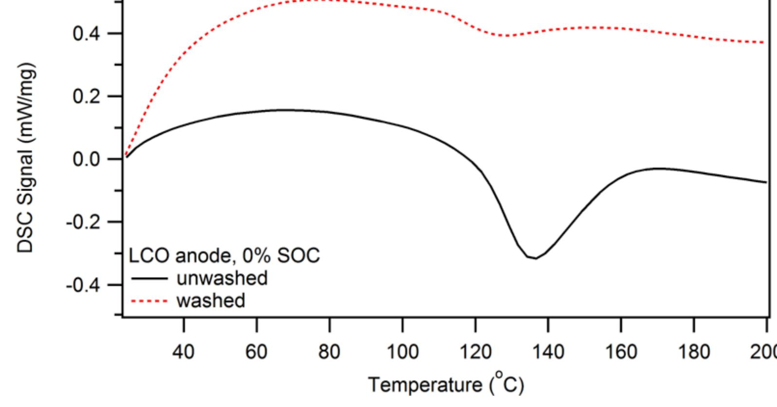
Exothermic peak is from metastable SEI + electrolyte decomposition. Washing the anode in DMC removes metastable SEI/electrolyte and also eliminates the exotherm.
