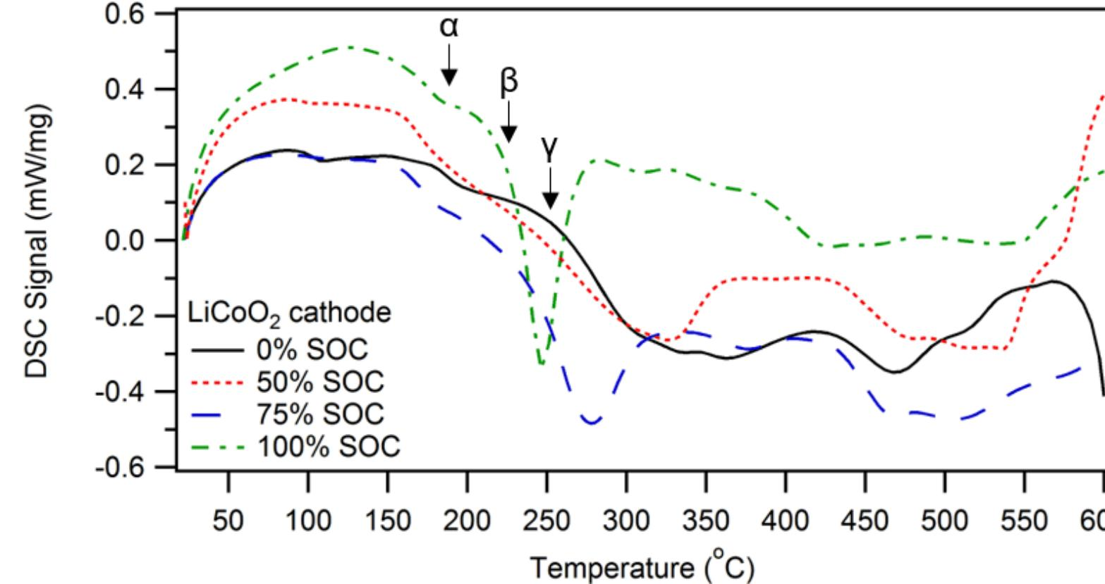
Exotherm onset ( $\alpha$ ) followed by a large peak ( $\beta$ ) at high SOC matches well ARC and XRD. Lower SOC have higher onsets ( $\gamma$ ) and minimal exotherm due to greater stability.
