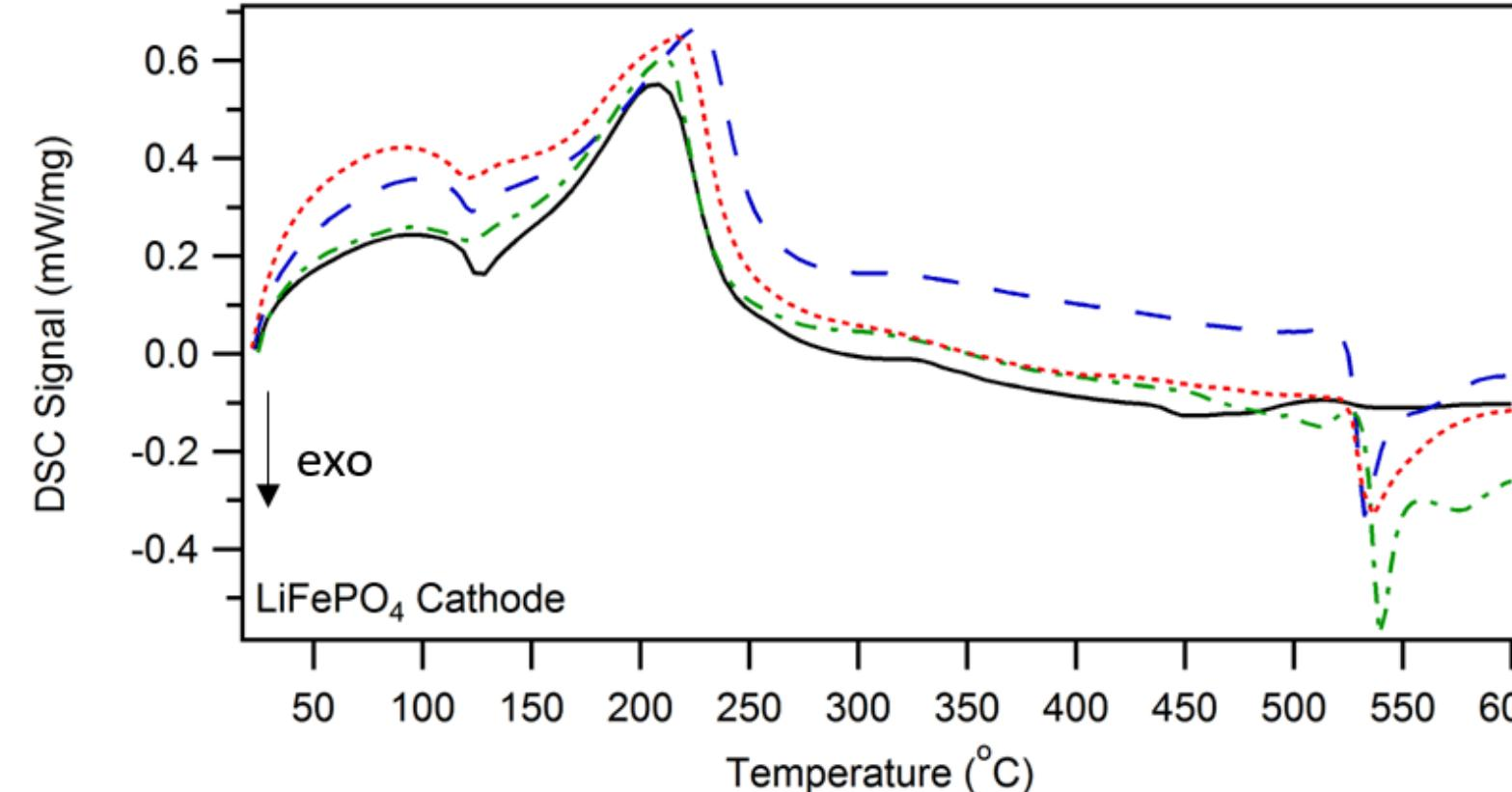
Cathode stable until > 500°C at all SOC, minimal exotherm noted. Endotherm exists 125-250°C, likely LiPF6/electrolyte decomposition. Cathode likely uninvolved in ARC response.
