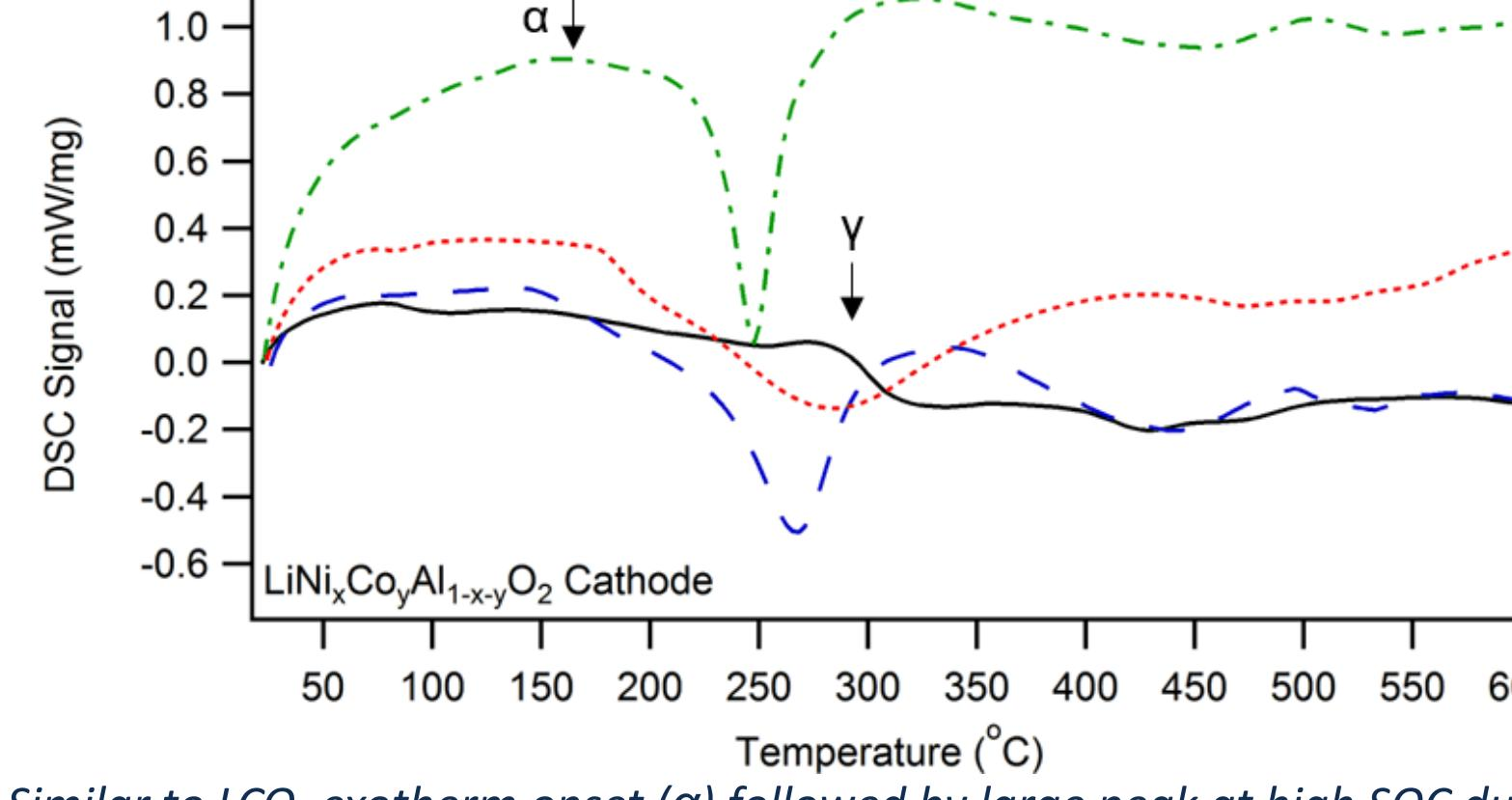
Similar to LCO, exotherm onset ( $\alpha$ ) followed by large peak at high SOC due to metastability of delithiated layered metal oxides. Lower SOC cathodes are stable ( $\gamma$ ).
