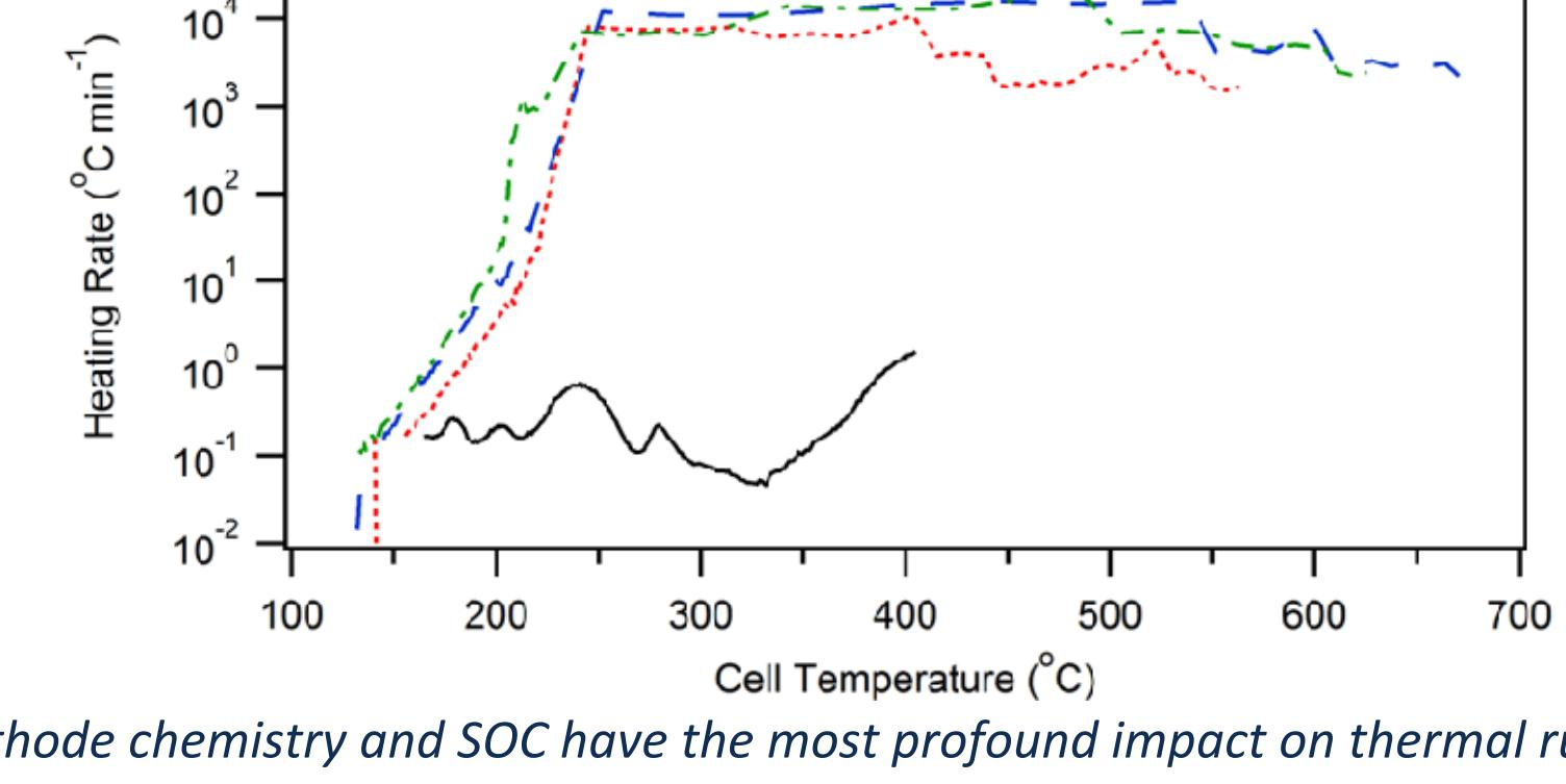
Cathode chemistry and SOC have the most profound impact on thermal runaway behavior, as they dictate  $HR_{max}$ .
