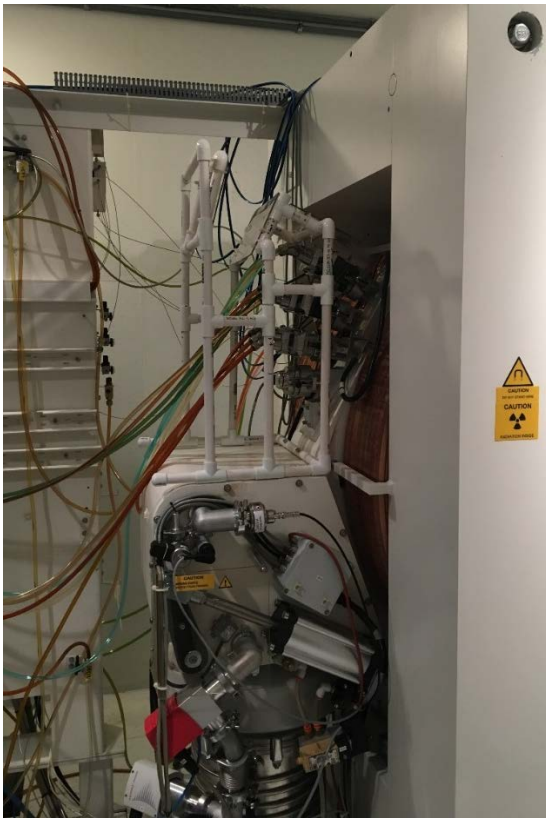
Figure 8: The MURR cyclotron (right) produced a proton beam to irradiate a 4 mL enriched water target ( ^1\text{H}_2^{18}\text{O} ), which behaved as an isotropic point source for neutrons.
