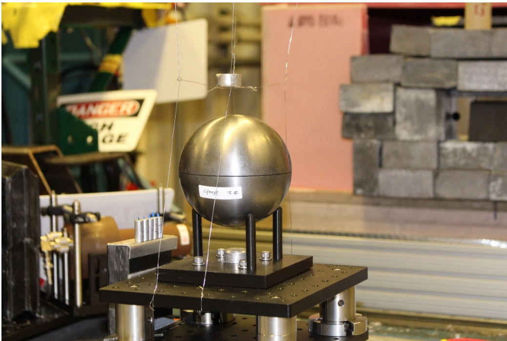
Figure 4: Indium pucks placed above and below the beryllium sphere. The indium pucks were 25 mm in diameter and 10 mm thick, while the beryllium sphere had an outer diameter of 11.3 cm.
