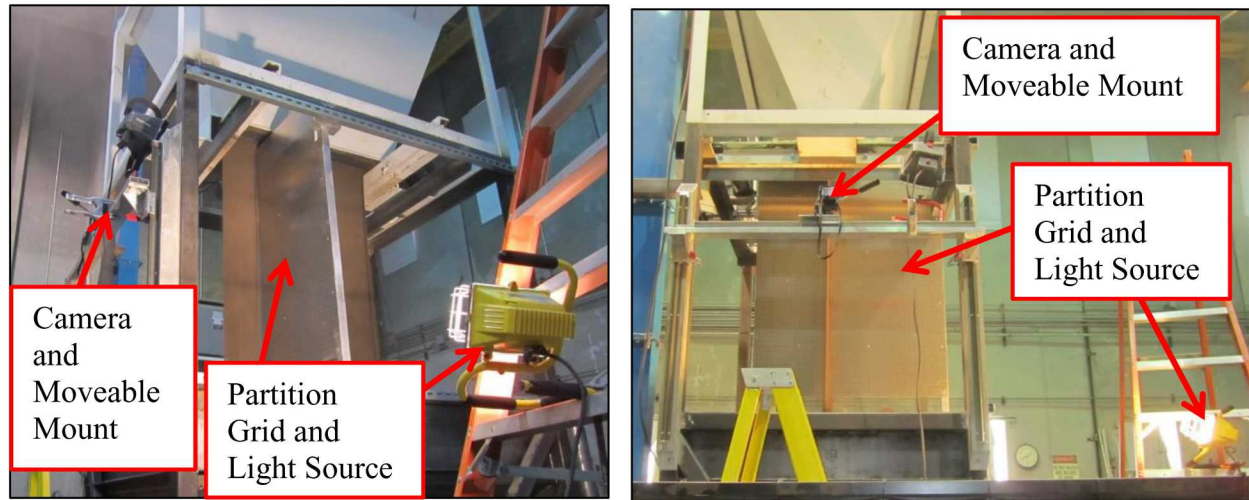
Figure 18. Left: Front-Side looking view of the particle curtain image system. Right: Side looking view of the particle curtain image system.
