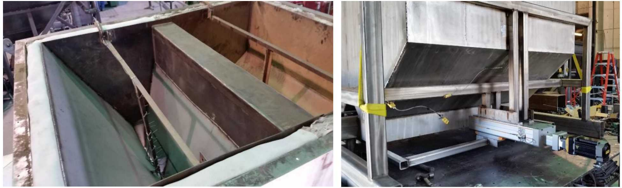
Figure 44. Left: Top hopper liner with steeper walls to enable more uniform particle mass flow along thermocouple tree. Right: Linear actuator mounted to the bottom of the top hopper to control the slide gate for particle mass flow control.
