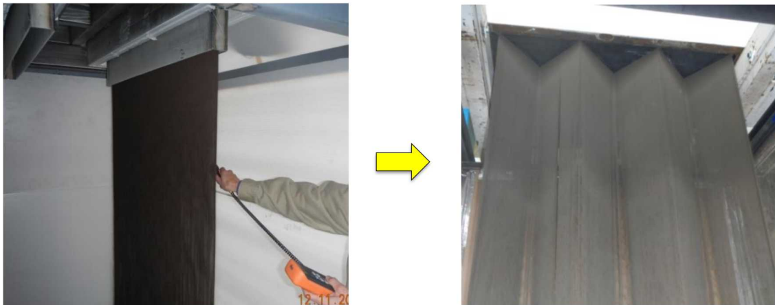
Figure 1. Left: particles dropped through a straight slot creating a planar “curtain” of falling particles. Right: Zig-zag particle release pattern for increased light trapping.
