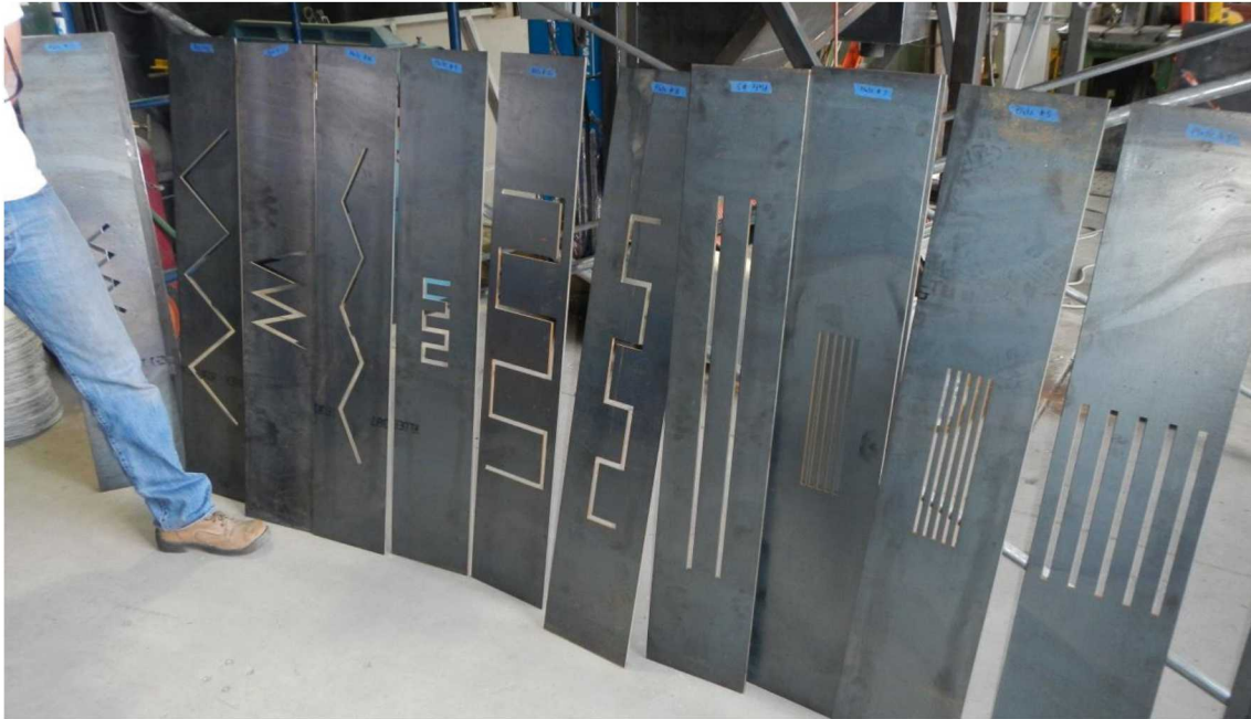
Figure 17. Different wave-like and parallel-line slot patterns machined into steel plates to evaluate alternative particle release patterns.
