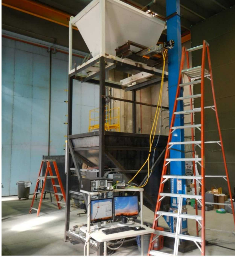
Figure 30. Control system and top hopper being tested under ambient conditions.
