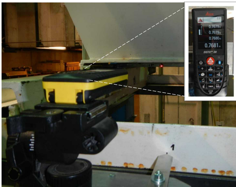
Figure 31. Measurement of the plate's leading edge using the Disto under ambient conditions. The red laser dot is visible on the leading edge of the plate.
