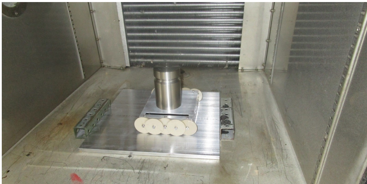
Figure 2.6.10. Robot chassis with wheels in ARL thermal chamber for thermal testing
