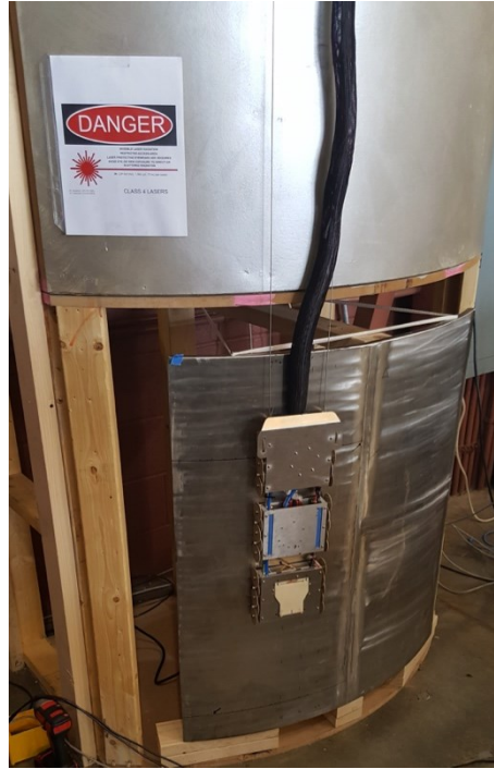
Figure 2.2.47. The sensor cars deployed onto the stainless steel canister mock up during the final technology demonstration at Test Track.
