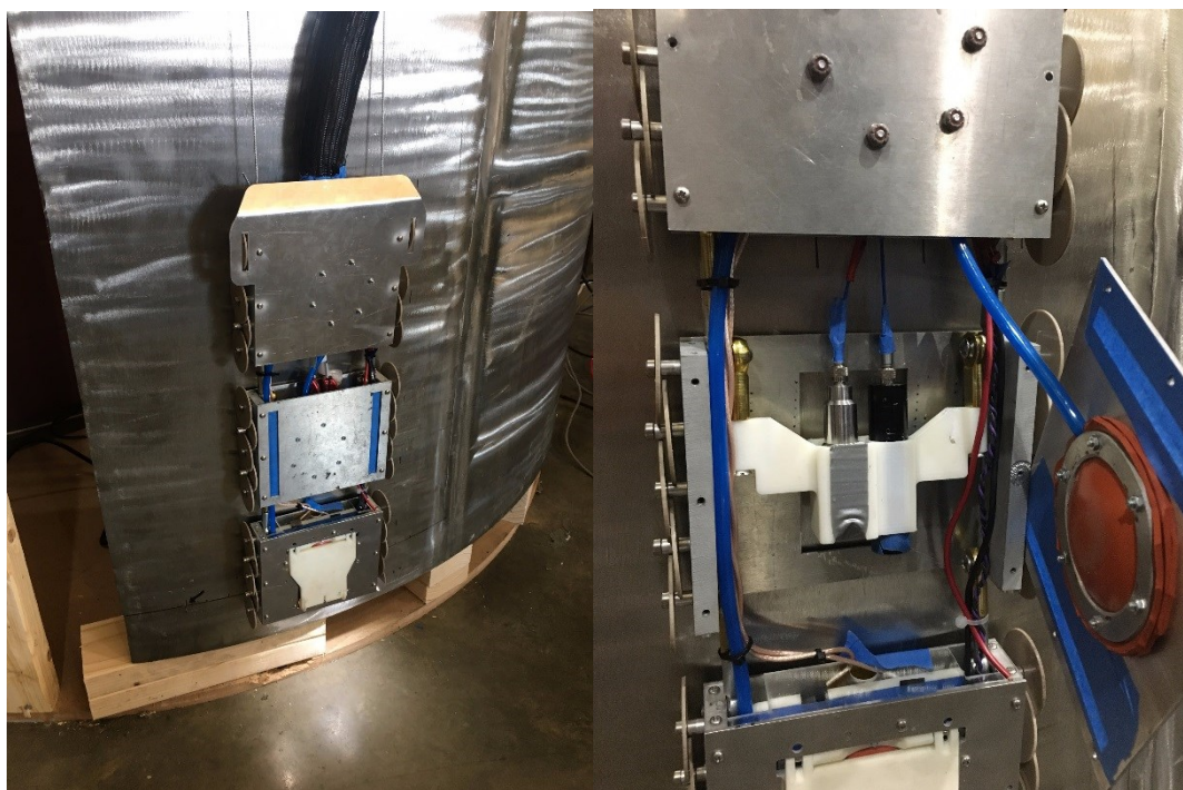
Figure 2.1.25. The LIBS optics holder mounted in the PRINSE robotic train. Operation of this system was tested once fully inserted into a simulated canister channel.
