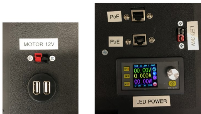
Figure 2.4.109. Labeled panel mount connections for winch and vent anchor cable bundles
