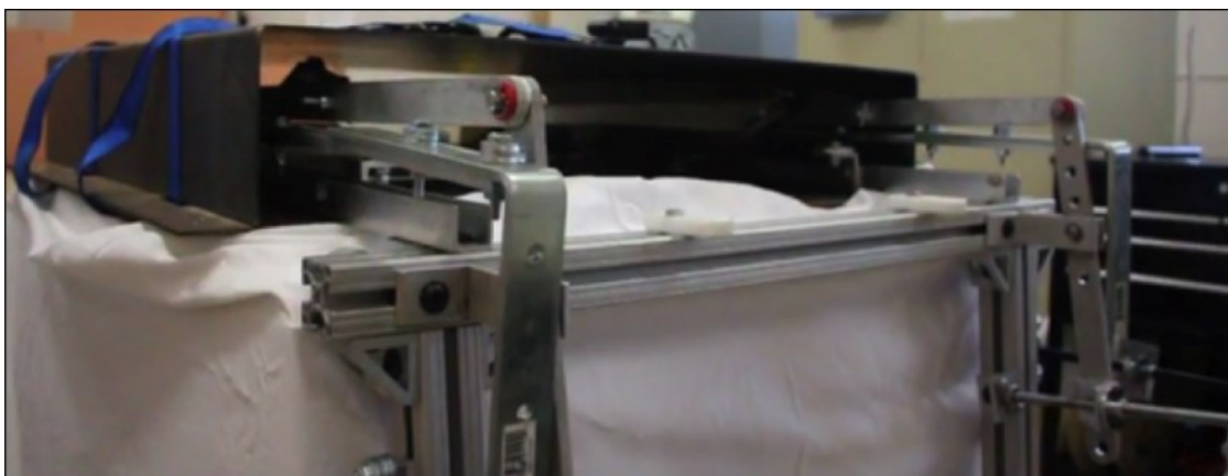
Figure 2.4.44. Vent anchor assembly inserted in vent opening
