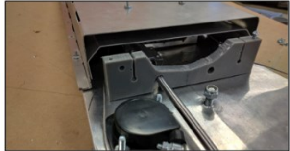
Figure 2.4.67. CAD concept and built version of garage with cable housing stops
