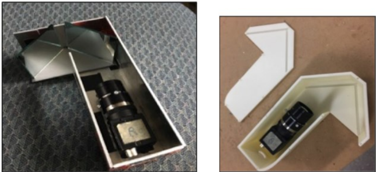
Figure 2.4.73. Aluminum and 3D printed camera box prototypes, showing the camera and two mirrors
