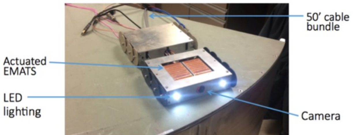
Figure 2.4.80. Bottom view of sensor car train showing camera, EMAT sensors, lighting, and cable bundle
