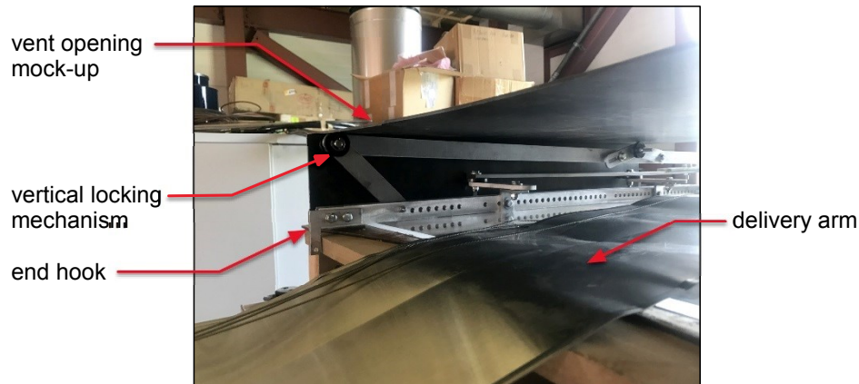
Figure 2.4.95. View of vent anchor inserted and locked into place from inside cask vent opening mock-up
