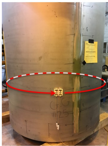
Figure 2.2.41. SH0 and SH1 waves travel around the MPC circumference many times.
