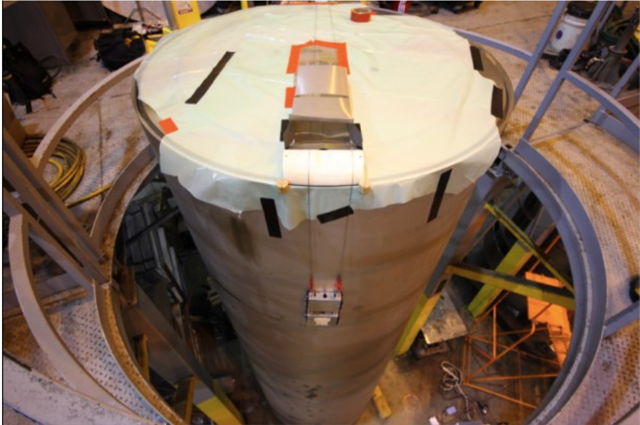
Figure 2.4.89. Delivery arm and sensor cars on the MPC at Holtec
