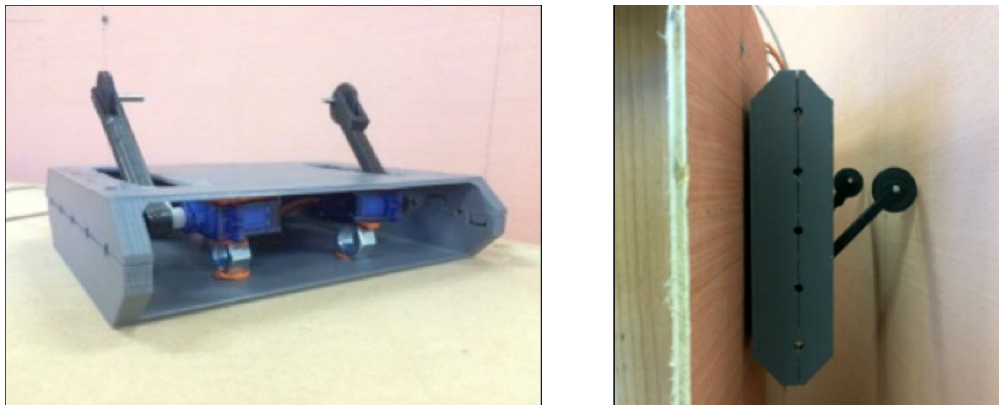
Figure 2.4.26. The first prototype stabilizing arms and servomotors
