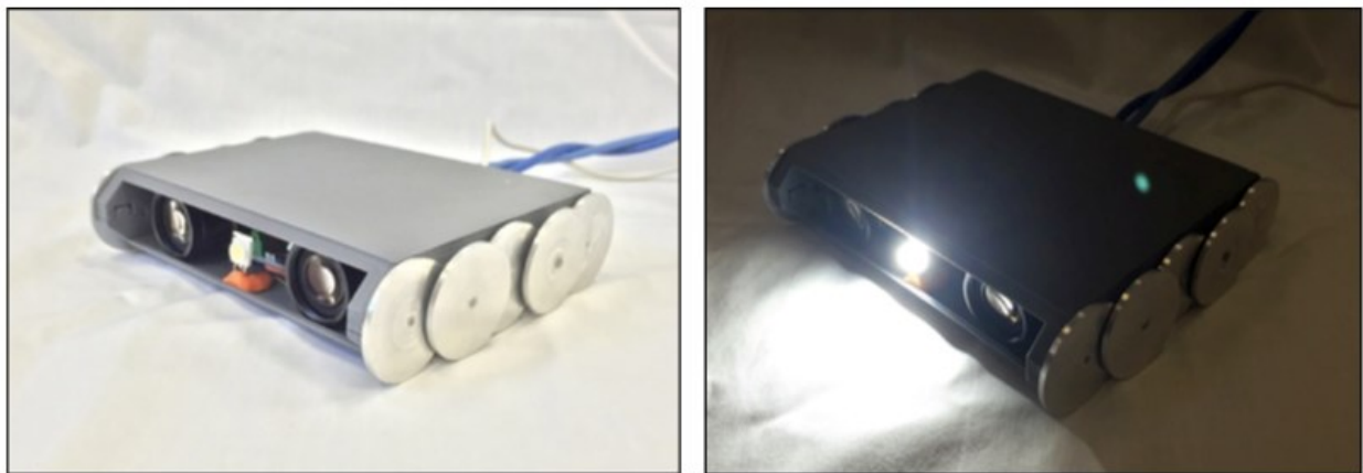
Figure 2.4.77. 3D printed sensor car prototype, showing camera lenses, LED, and wheels
