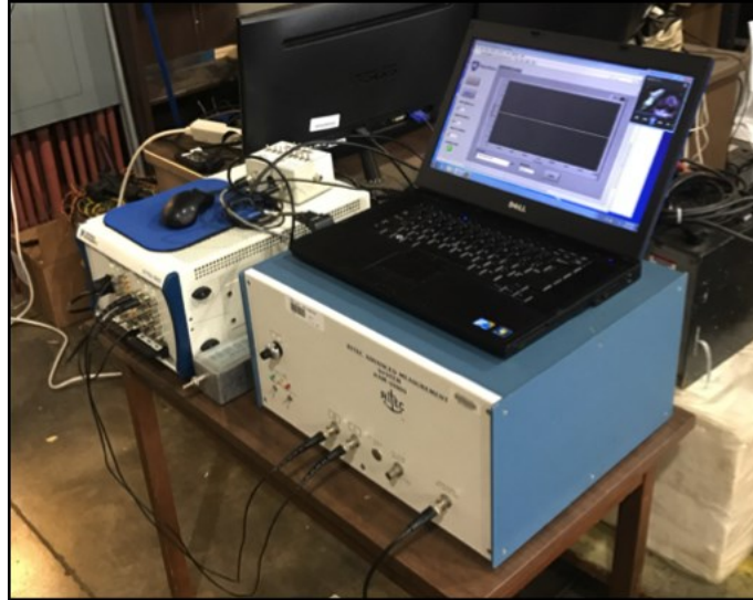
Figure 2.2.11. Desktop command center instrumentation; Ritec amplifier, NI controller, laptop.
