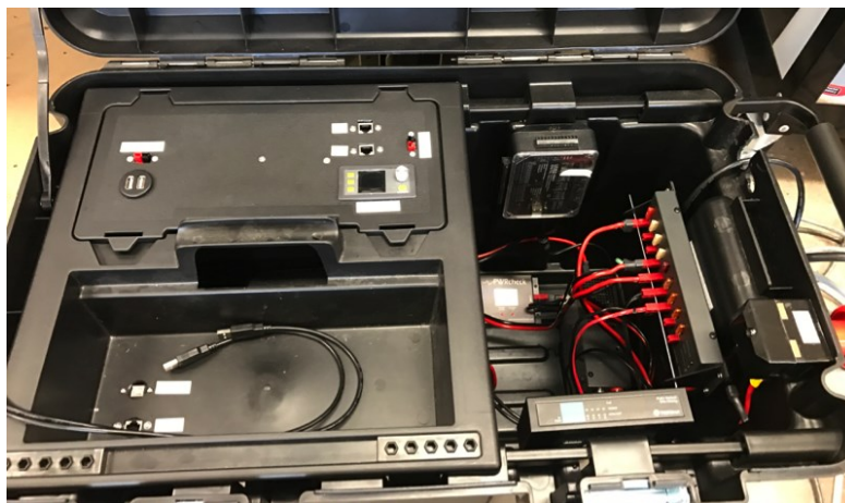
Figure 2.4.107. Interior of power supply box; deep cycle battery is below the tray on the left
