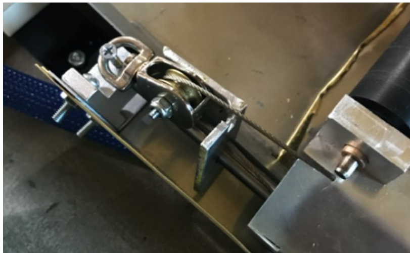
Figure 2.4.72. Pulley for pushing mechanism cable
