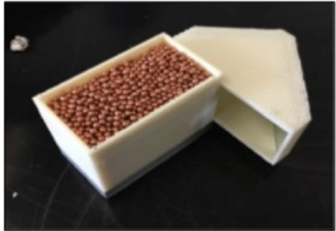
Figure 2.4.74. Exploded diagram (left) and completed 3D printed camera box prototype filled with lead shot (right)
