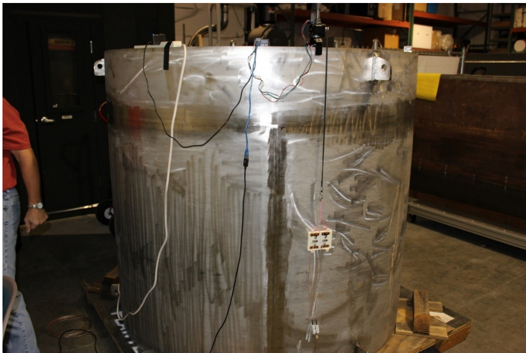
Figure 2.2.43. Full-diameter partial height canister mockup with EMAT pair on the right side of the 4 ft long axial weld.
