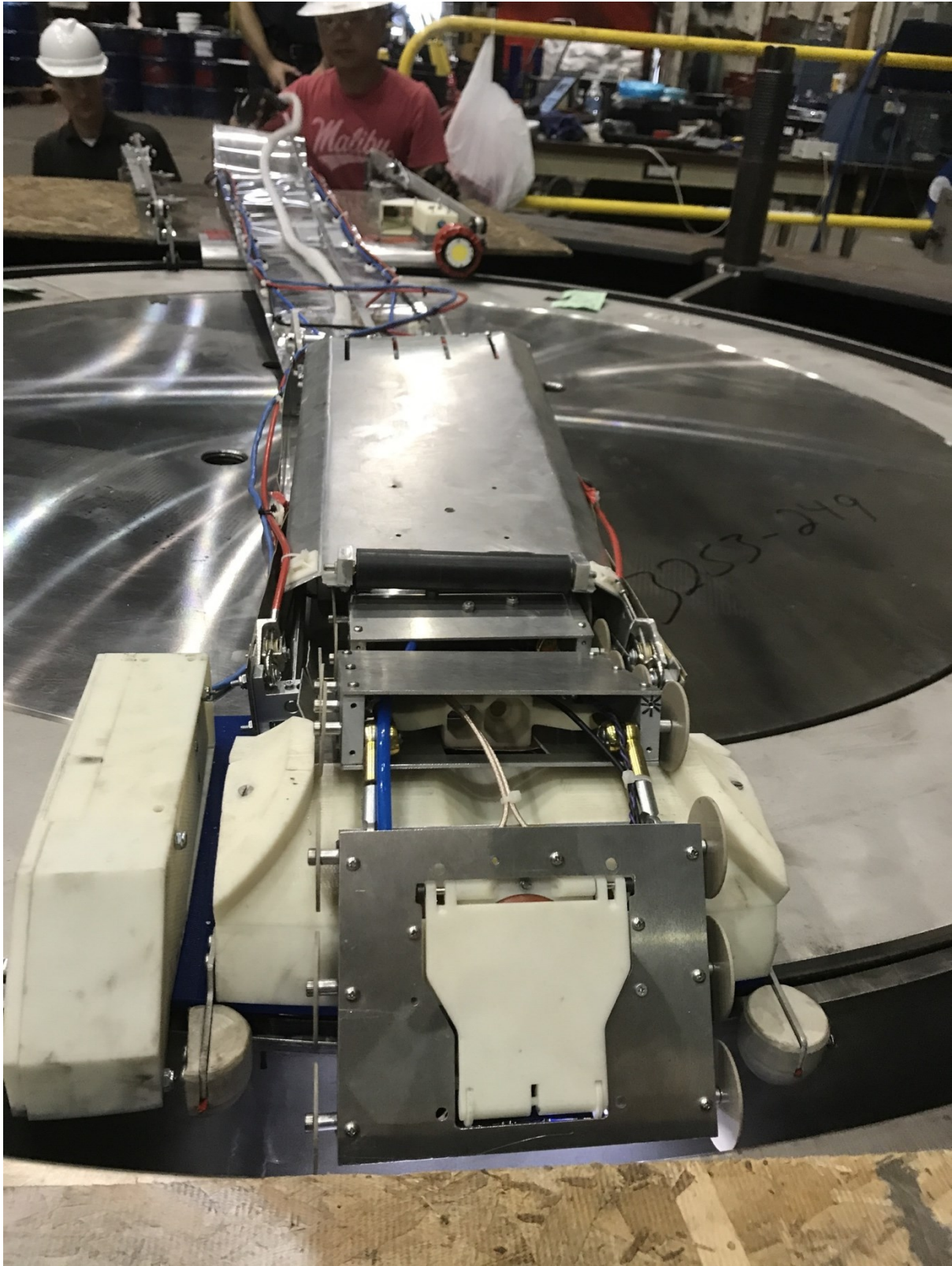
Figure 2.7.4. Sensor car 1 pulling car 2 over the hump.
