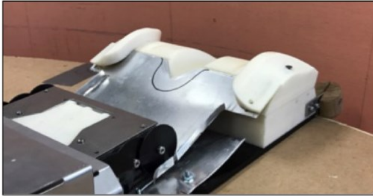
Figure 2.4.64. 3D printed delivery arm end guide structure installed on delivery arm, with sensor cars in garage.
