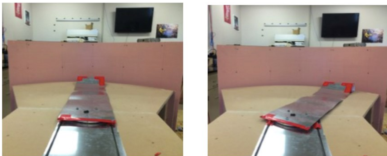
Figure 2.4.59. The pivoting delivery arm prototype in two different positions
