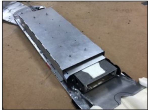
Figure 2.4.64. 3D printed delivery arm end guide structure installed on delivery arm, with sensor cars in garage.
