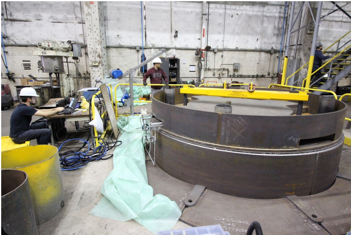
Figure 2.7.1. Cask in pit – vent bracket installed in one outlet vent and command station setup on left side.
