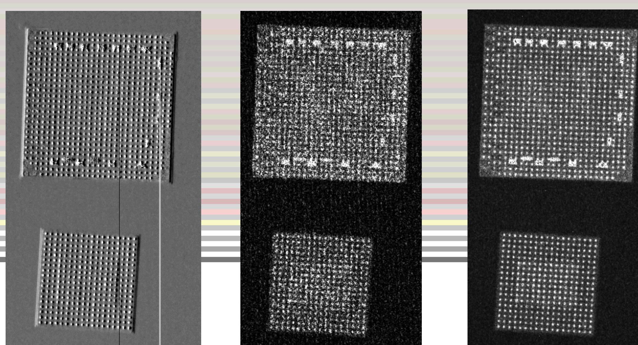
**Left:** Fourier domain processed differential phase image product: streaks are columns lost from unsuccessful phase unwrapping with a 1D algorithm.
