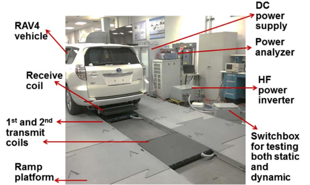
Fig. 10. Stationary and dynamic wireless power transfer laboratory test setup.
