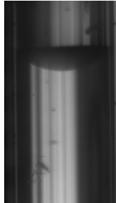
Contact angle measurement Left: non-wetting on printed channel (middle), and wetting contact angle on glass capillary
