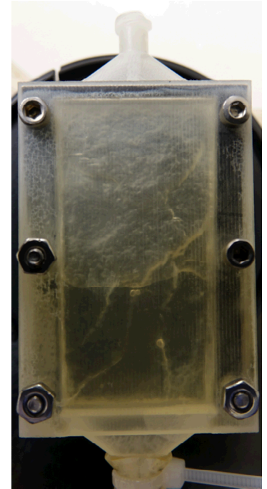
3D printed sample of single fracture (sealing unit is also printed)
