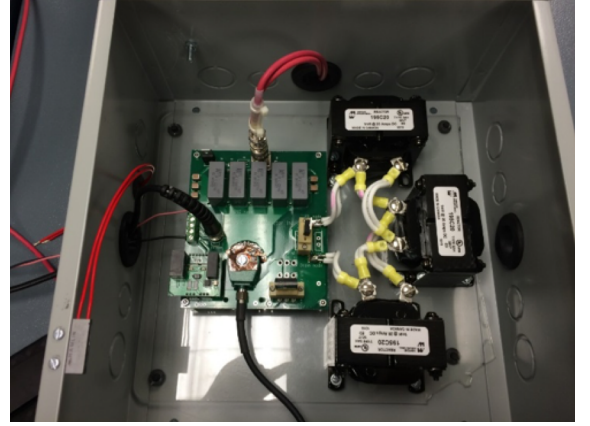
Fig. 7. Photograph of DPTC used for switching stress of the v-GaN diodes.
