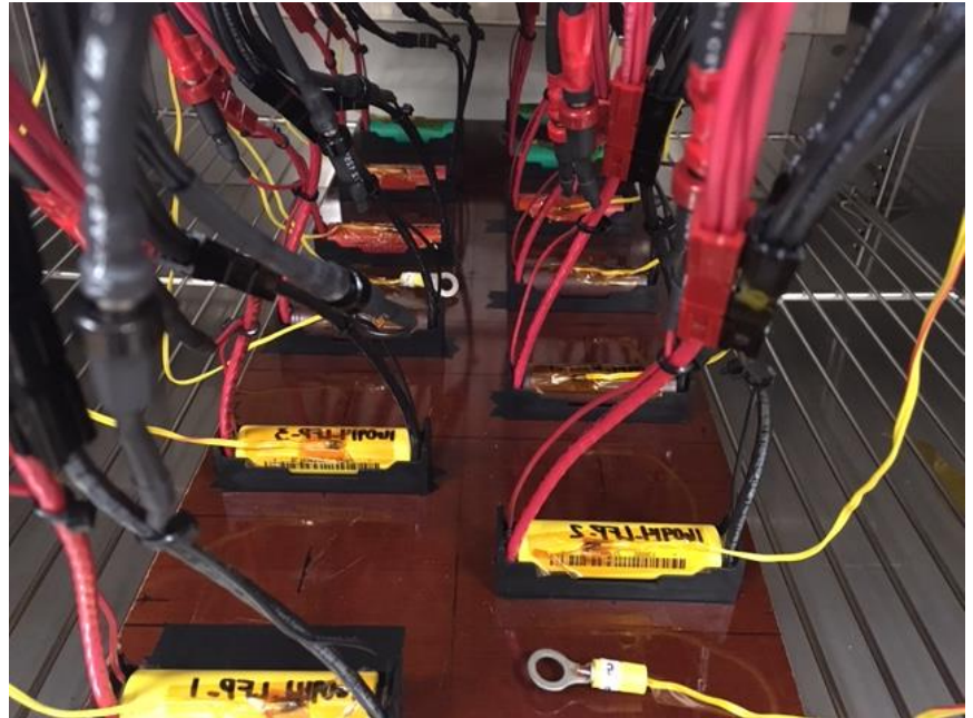
Li-CoO 2 Batteries under testing condition
