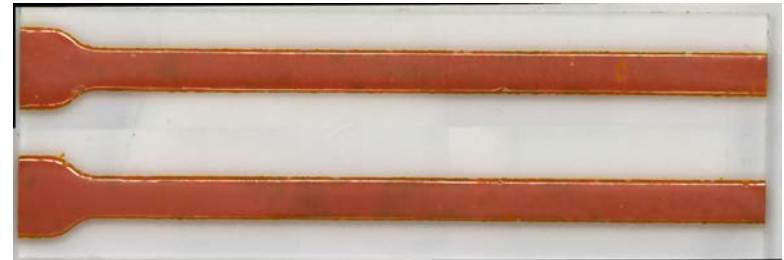
Photograph of HNAB films on 1 × 3 cm polycarbonate substrates. During deposition, a mask was used to define two film widths of 400 and 1600 \mu\text{m} .
