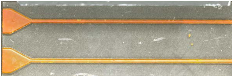
Photograph of HNAB films on 1 × 3 cm polycarbonate substrates. During deposition, a mask was used to define two film widths of 400 and 1600 \mu\text{m} .
